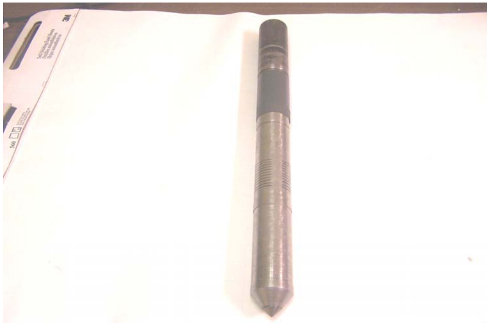
Figure 3-9 Probe tip closed for horizontal flow
