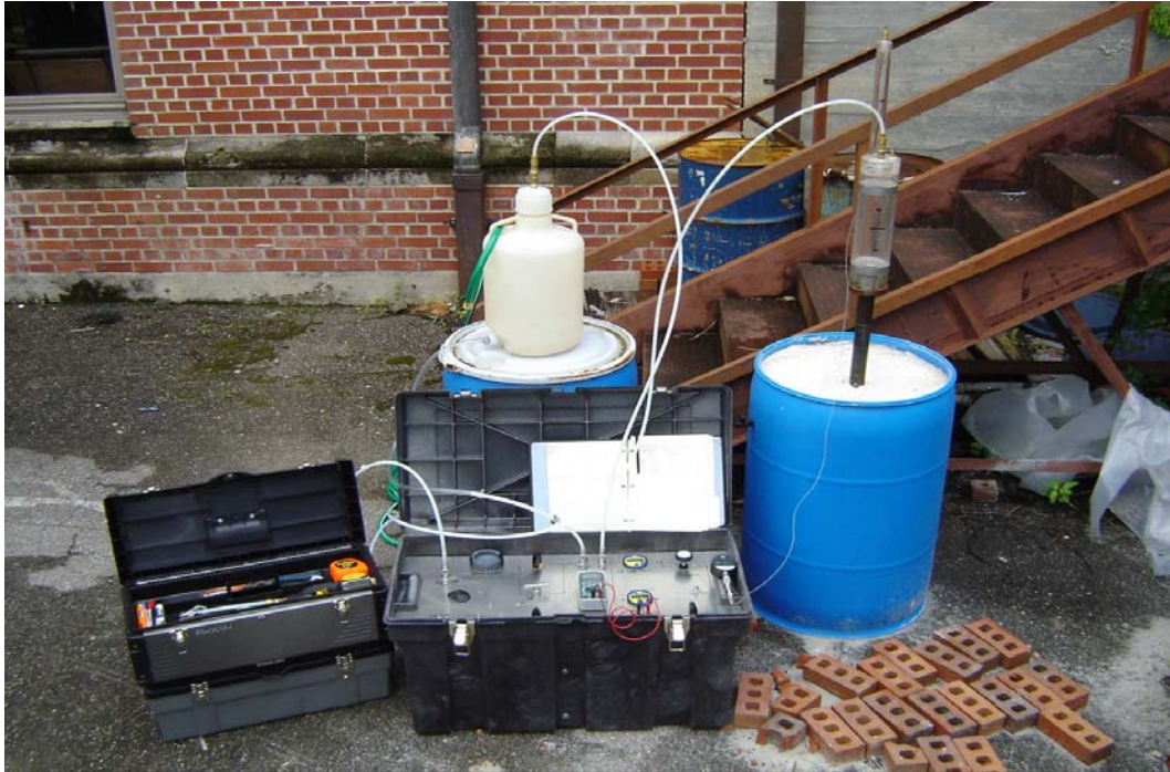
Figure 5-2 Setup for Sand Barrel Test
