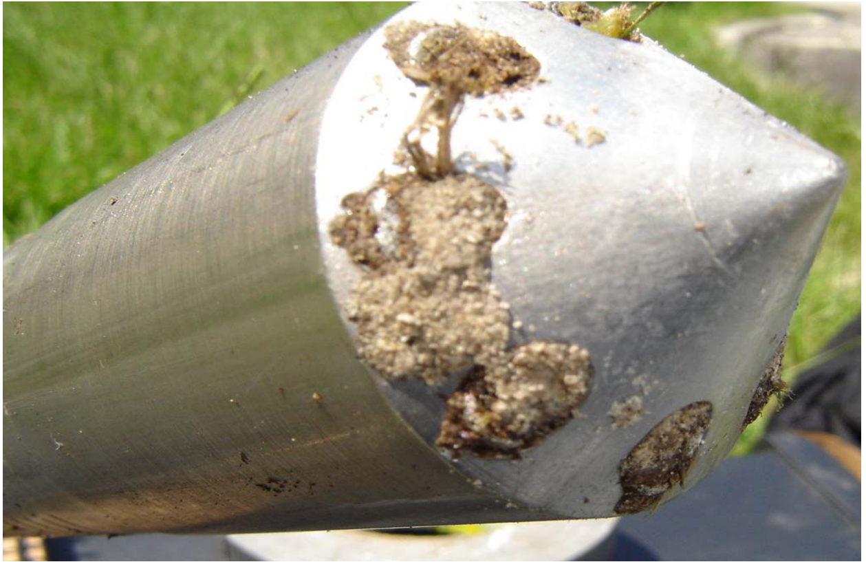
Figure 3-6 Potentially clogged flow ports (2005 probe)
