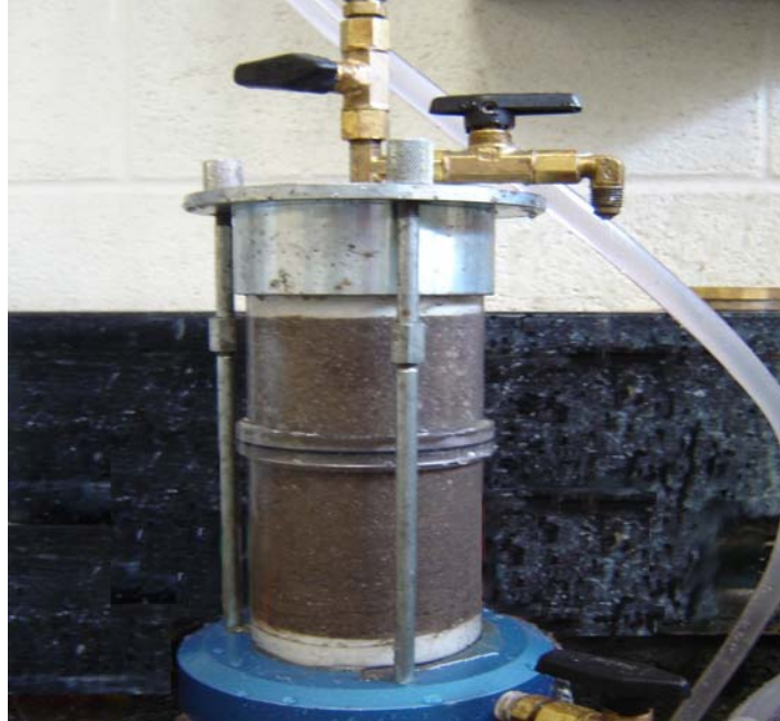
Figure 5-7 Laboratory permeability test on sample
