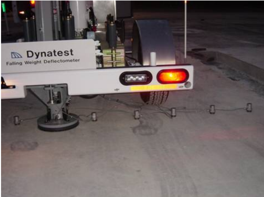
Figure 5.20. FWD Test at the Center and Measuring Deflections Along the Transverse Center-Line.
