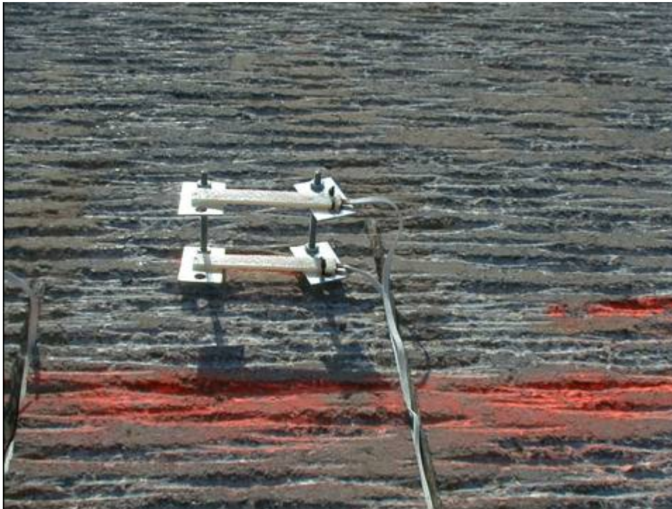
Figure 3.16. Placement of Top and Bottom Strain Gages on Lane 7 in Phase I-b.
