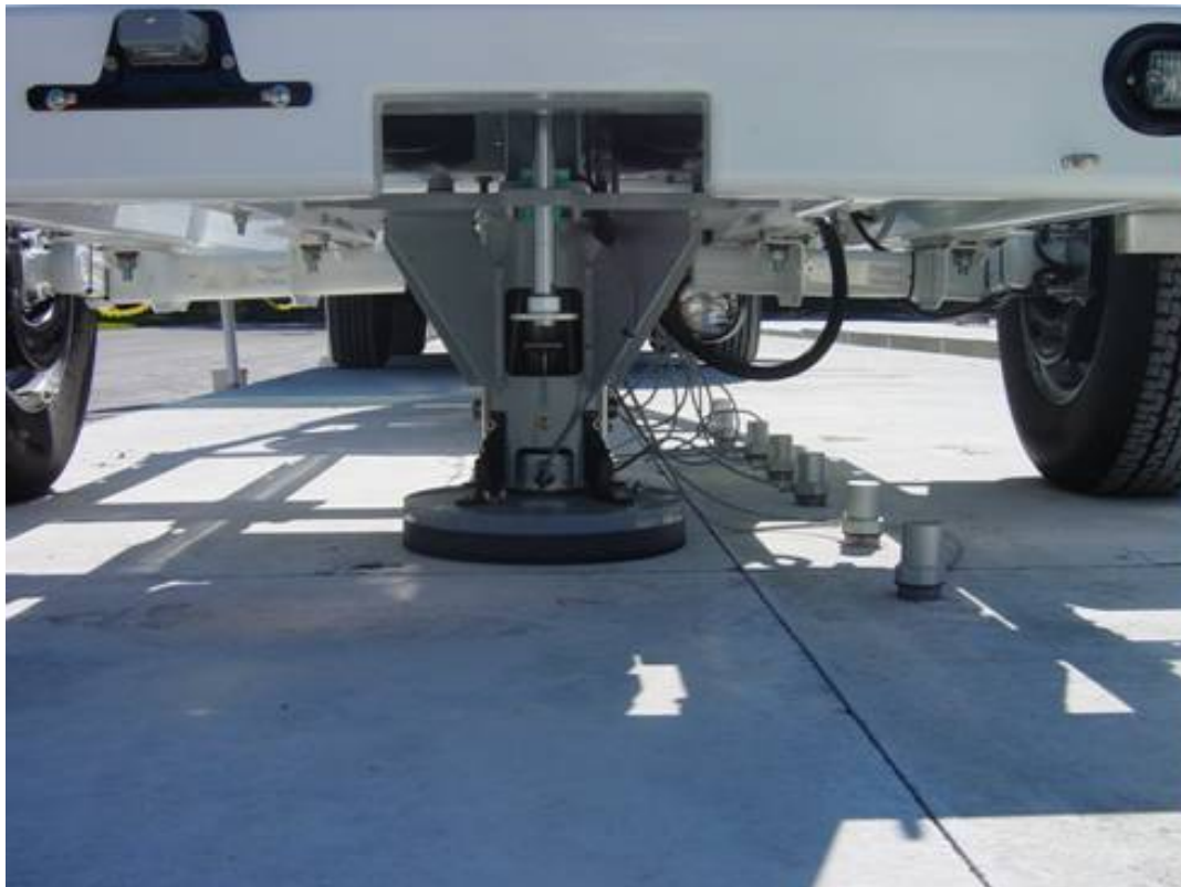
Figure 5.18. FWD Test at the Slab Corner and Measuring Deflections on the Opposite Slab.
