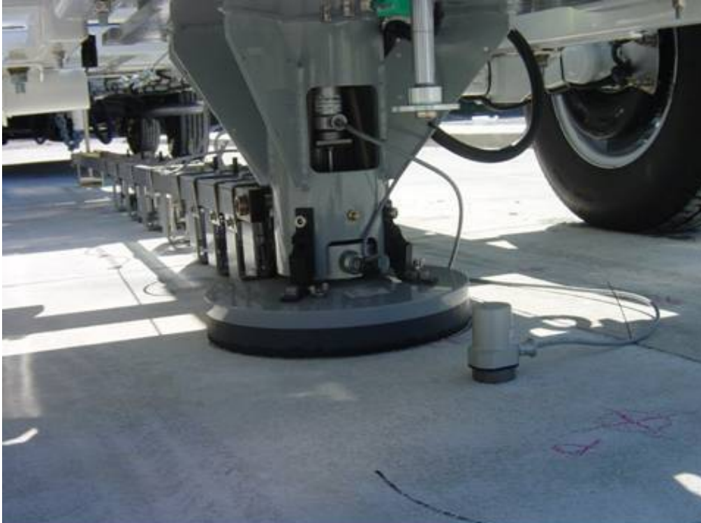
Figure 5.19. FWD Test at the Mid-Edge and Measuring Deflections in the Loaded Slab.
