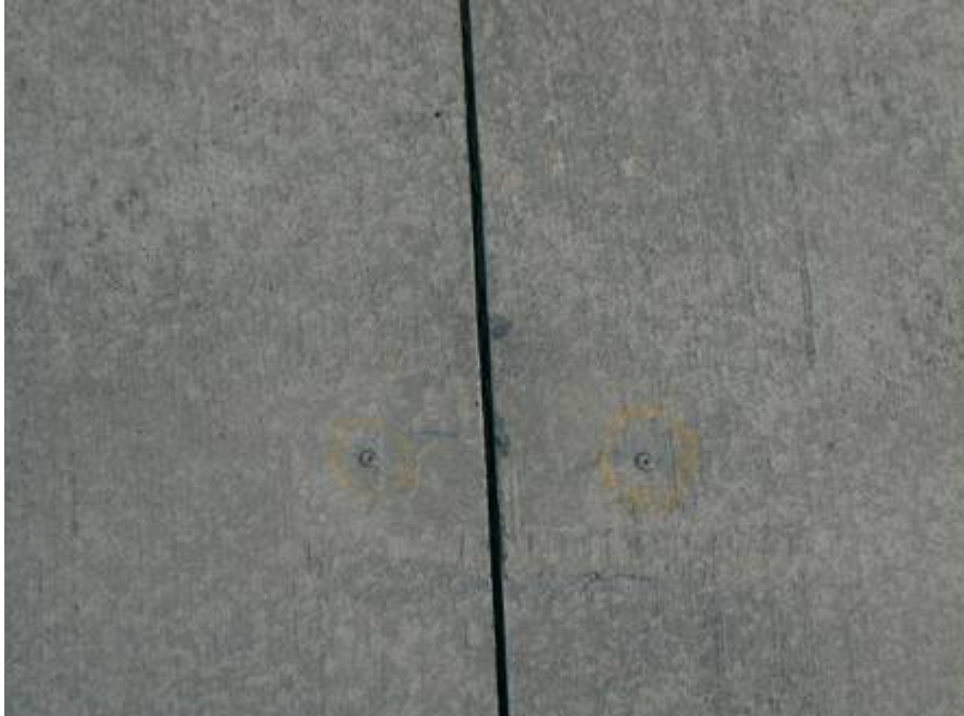
Figure 5.4. A Pair of Whitmore Plugs Fixed at a Joint.
