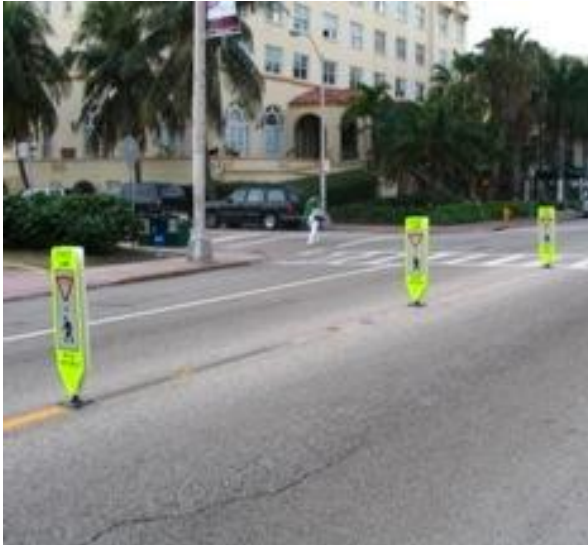
Figure 3.8 Picture of In-street “Yield to Pedestrians” Signs
