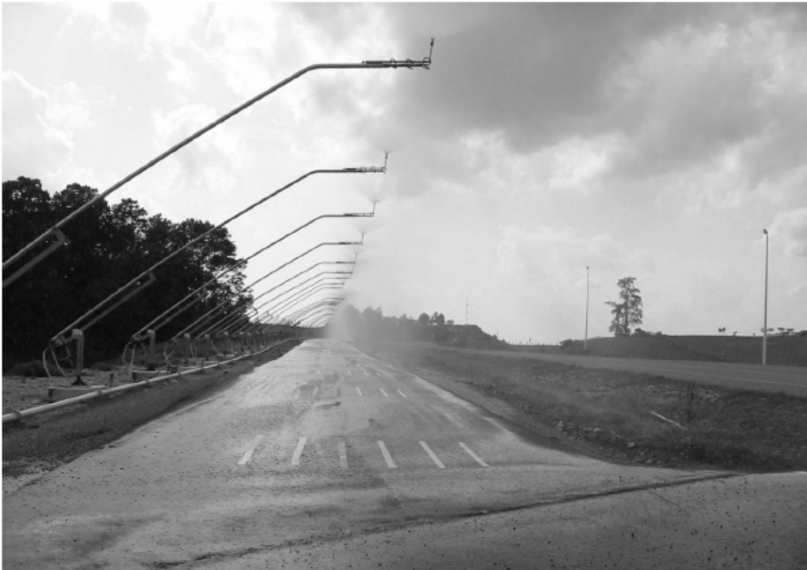
Figure 3-3. Rain Simulation System Used in VTTI Study (6)
