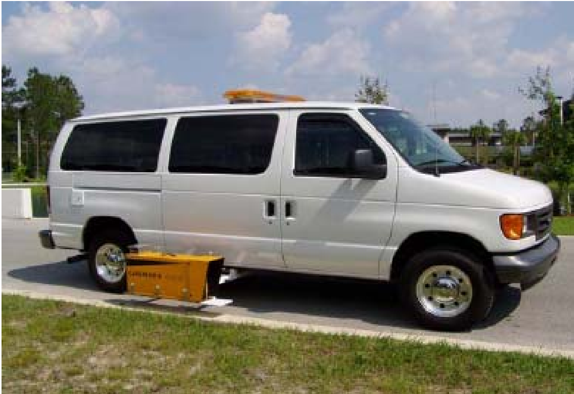
Figure 2-1. FDOT Van with Laserlux Attached (13)
