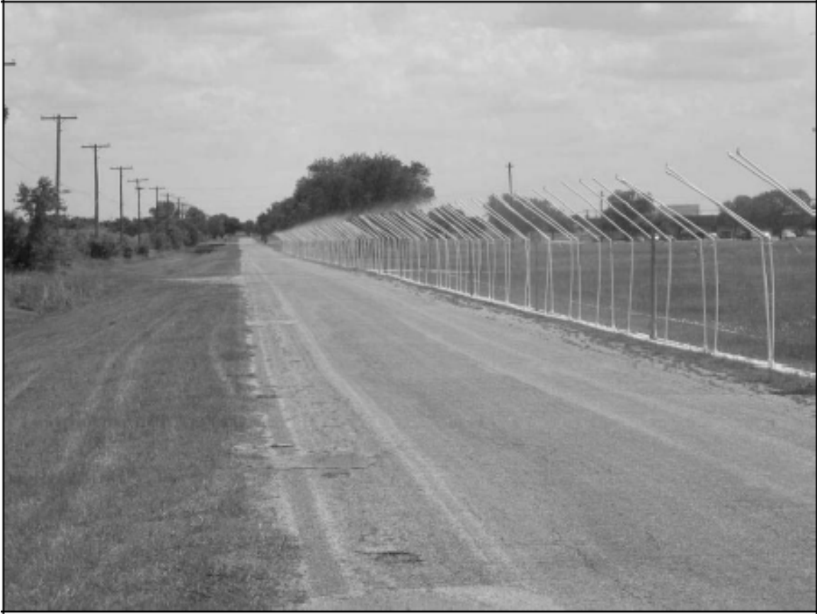
Figure 3-4. Rain Tunnel Used in TTI Study (8)
