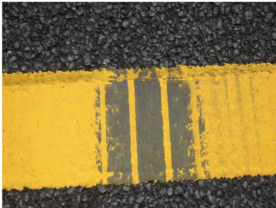
Figure 3-4. Wheel Tracking of Asphalt on to Surface of Pavement Marking (Product: E, Color: Yellow, Glass Beads: No)
