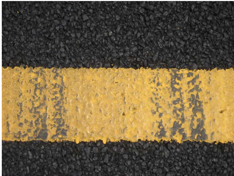
Figure 3-2. Wheel Tracking of Asphalt on to Surface of Pavement Marking (Product: D, Color: Yellow, Glass Beads: No)
