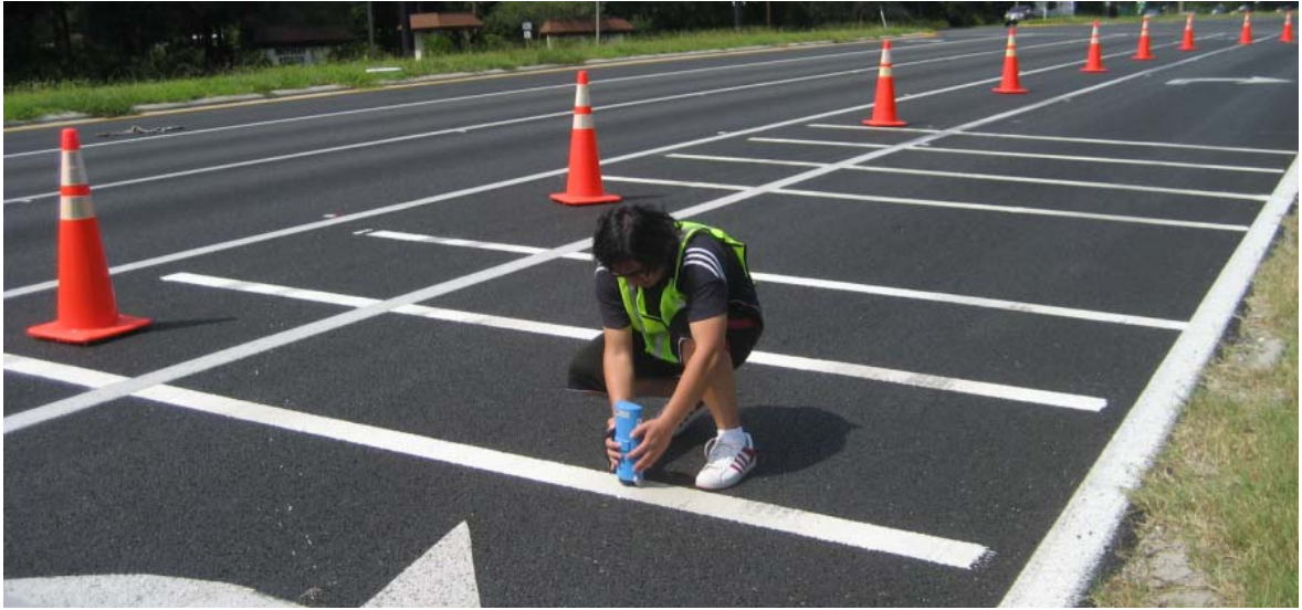
Figure 2–3. Measure Color using a BYK Gardner Handy Color.
