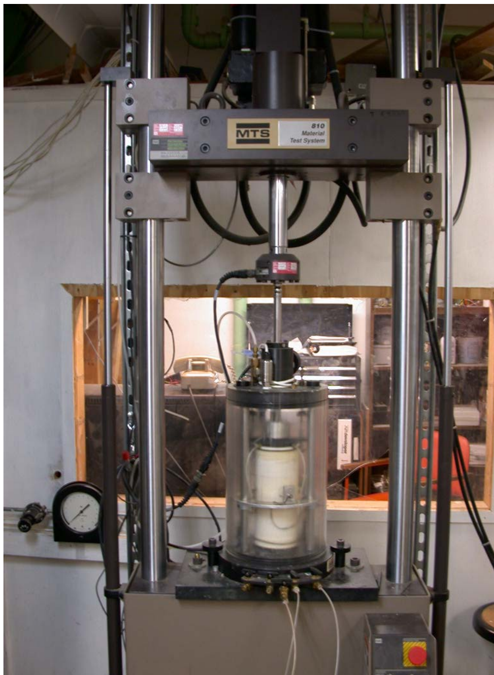
Figure 3.2 Resilient Modulus Test Setup
