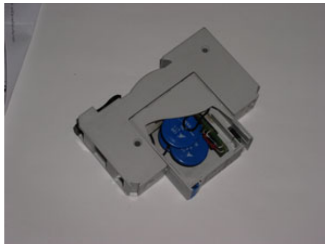
Figure 12. Damage to CITEL DS210-12VDC Suppressor
