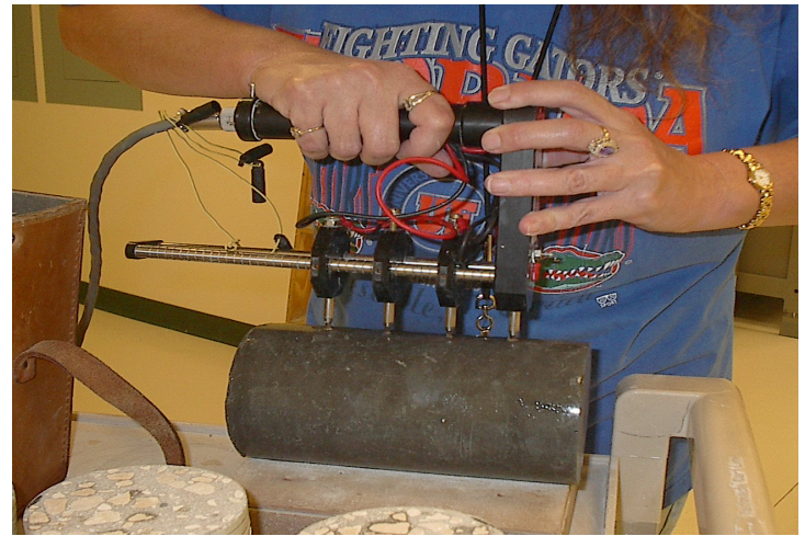
Surface resistivity test conducted on a concrete cylinder. SR is a rapid, nondestructive method to estimate long-term concrete permeability.
