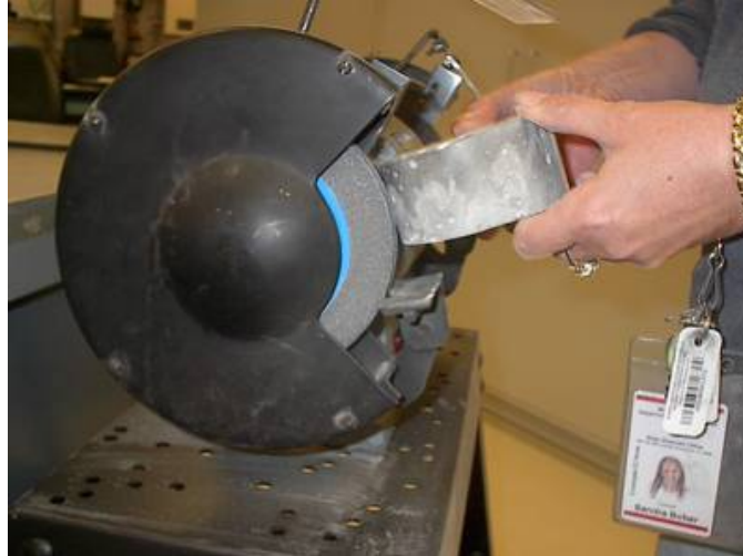
Figure 16. Preconditioning RCP Sample Surfaces to Receive Epoxy.
