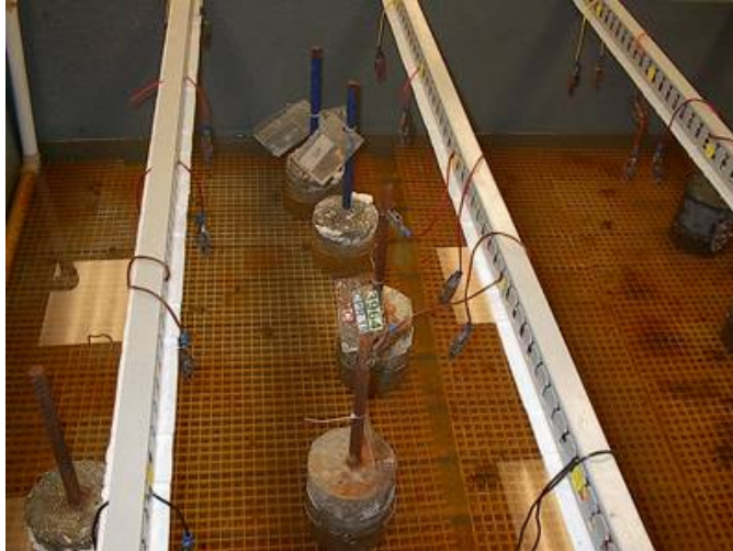
Figure 30. Impressed Current Test Set-up.
