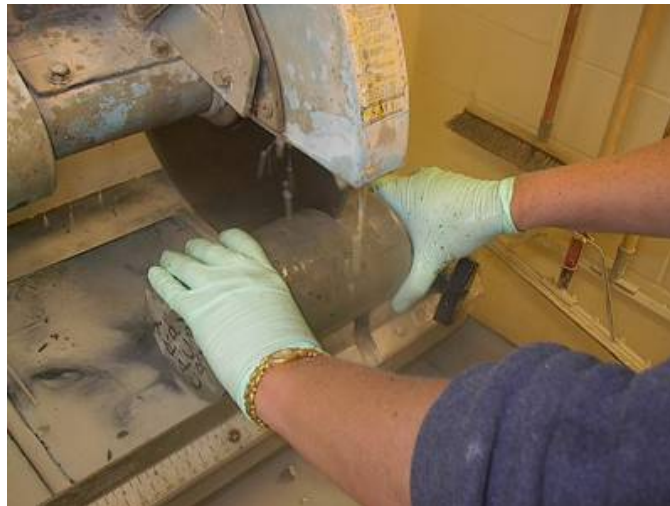
Figure 15. Cutting of the 2-inch Sample for the RCP Test.
