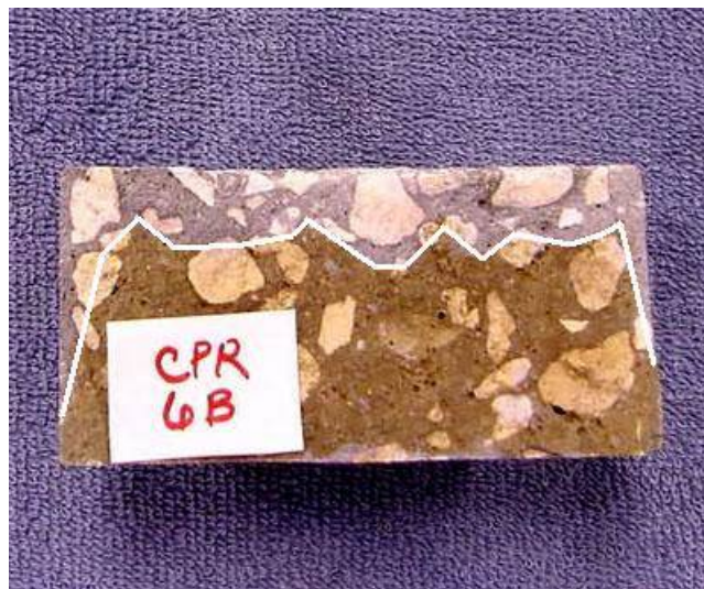
Figure 26. Split Surface of the Specimen Sprayed with the Silver Nitrate Solution.
