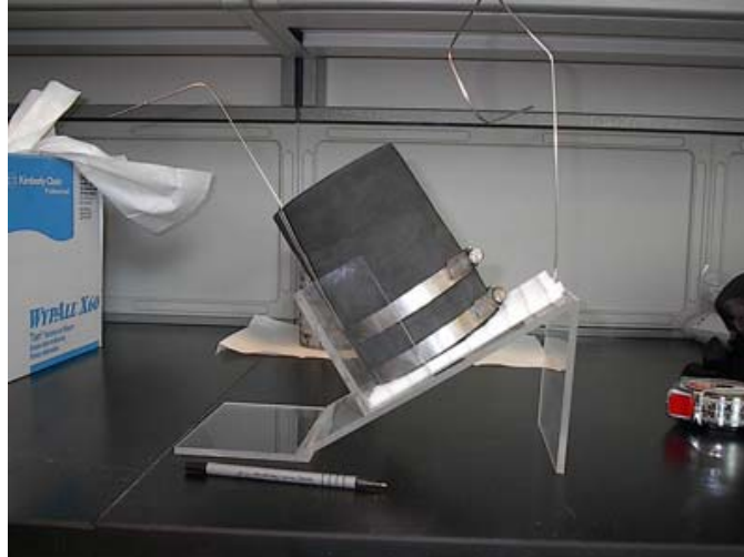
Figure 23. RMT Test Set-up shown prior to being immersed in the catholyte solution.
