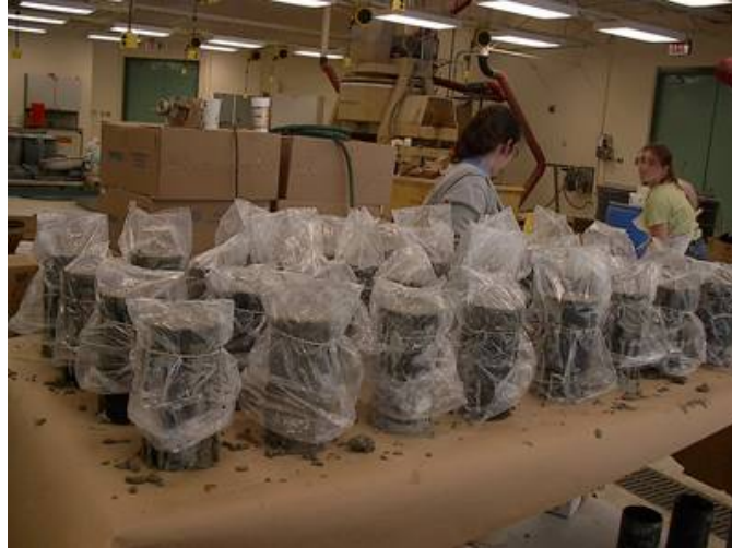
Figure 8. Air Curing of Cast Concrete Specimens.
