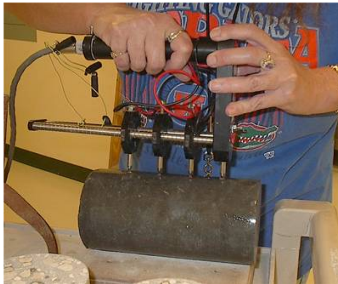
Figure 29. Surface Resistivity Measurements.
