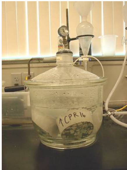
Figure 19. RCP Sample Desiccation.
