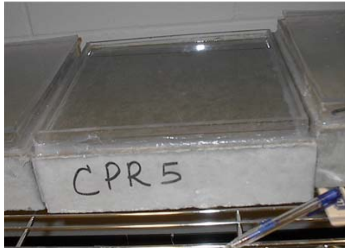
Figure 12. Ninety-day Salt Ponding Test Set-Up used in CPR
