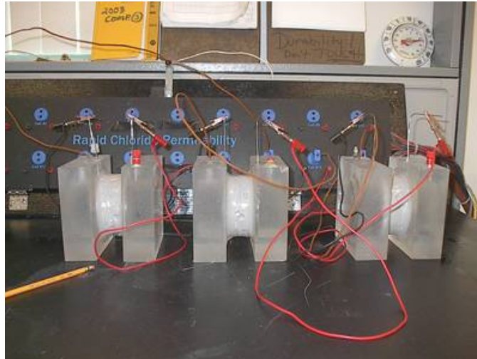
Figure 20. RCP Test Set-up.
