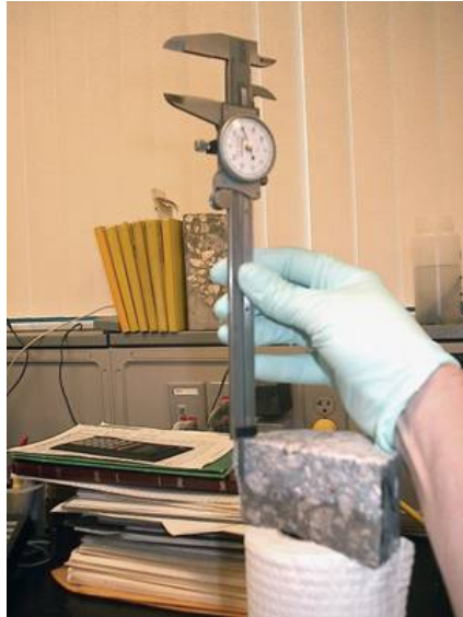
Figure 27. Chloride Penetration Measurement using the Silver Nitrate Solution Method.
