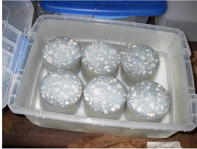
Figure 13. Bulk Diffusion Saline Solution Exposure.
