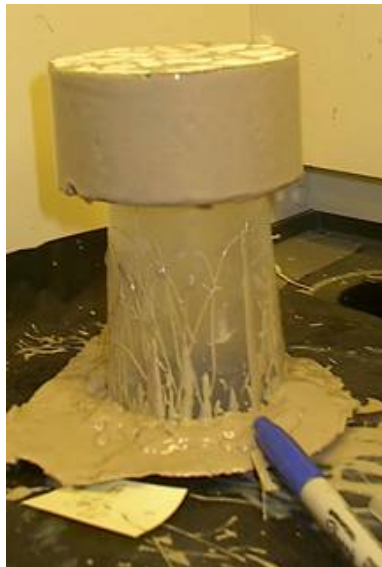
Figure 17. RCP Sample Sealed with Epoxy.
