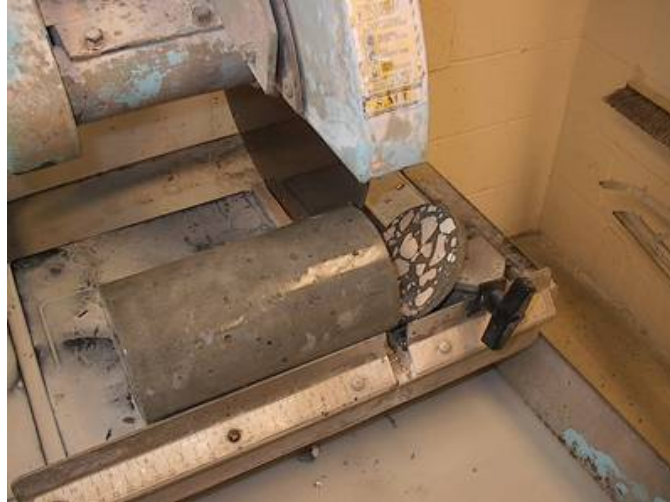
Figure 14. RCP test top surface removal of the sample preparation procedure.
