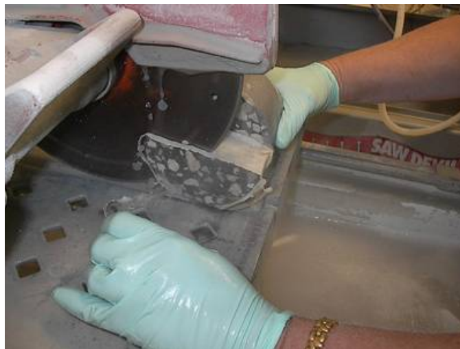
Figure 28. Slicing Samples for Comparison between FM 5-516 and Silver Nitrate Solution Spray Chloride Methods.
