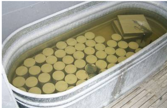
Figure 10. Field Samples Curing during transport to Laboratory.
