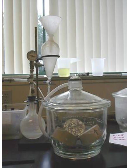
Figure 18. RCP Reduction of Absolute Pressure for Sample Desiccation.
