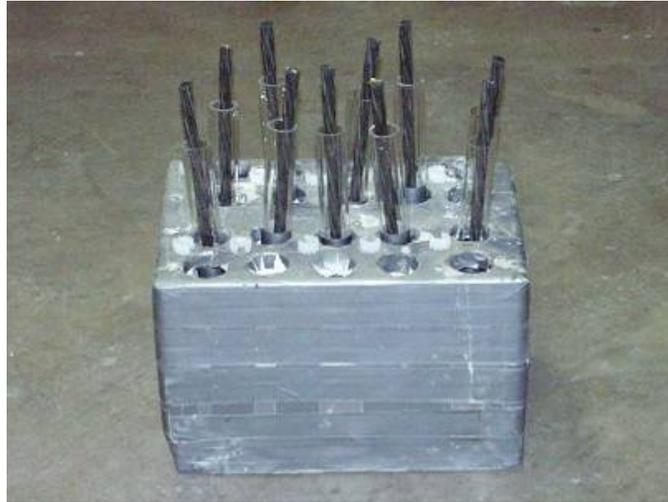
Figure 21 - Set of casings with placed strands ready for the casting procedure
