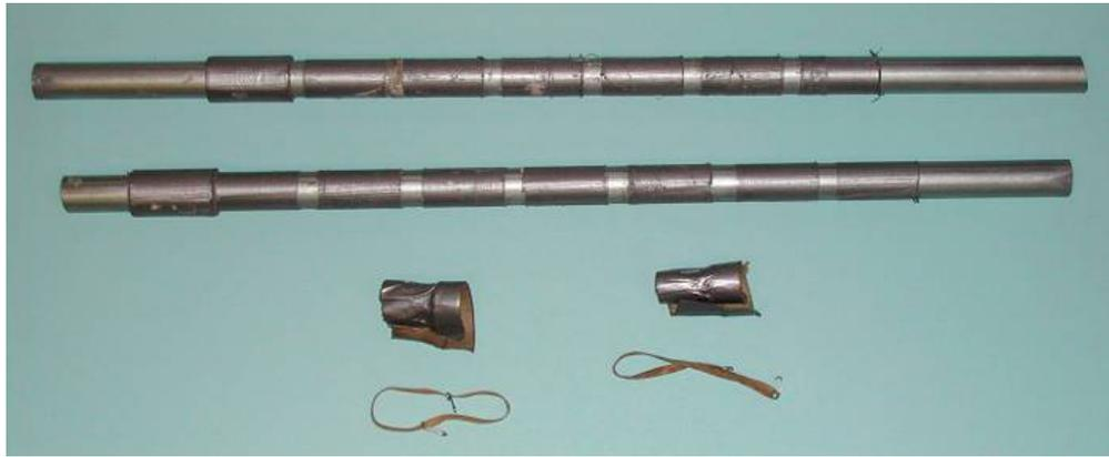
Figure 19 – Auxiliary tubing supports used in the assemblage of the ACT casings
