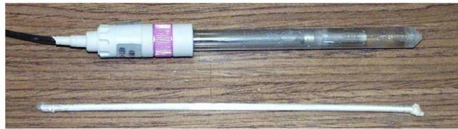
Figure 27 - Reference and counter electrodes used
