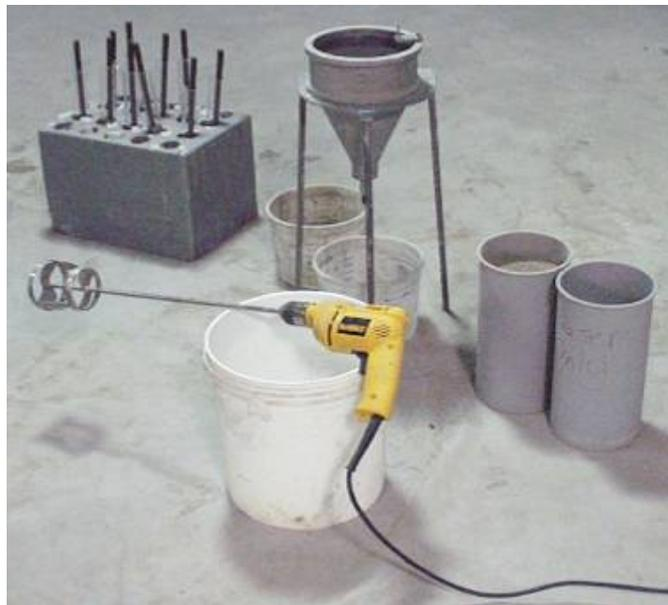
Figure 22 - Grout mixing and specimen casting ready to begin
