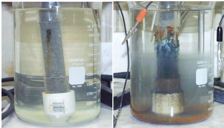
Figure 14 - Volume of corrosion products for low and high level of currents
