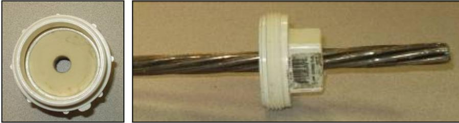
Figure 74 – Wick pressure test base cap and strand positioning.
