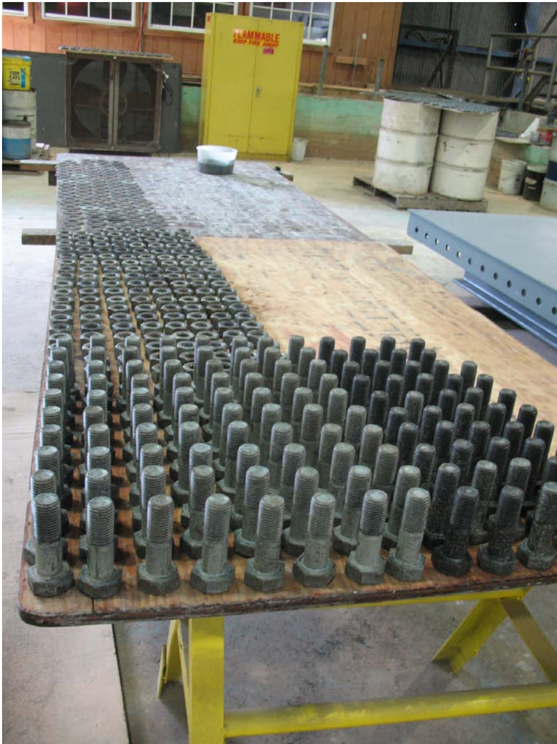
Figure 38. Bolts and nuts being cleaned and painted.
