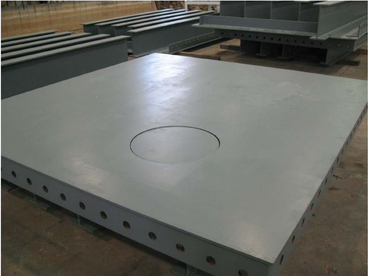
Figure 40. Side panel showing pipe access port.
