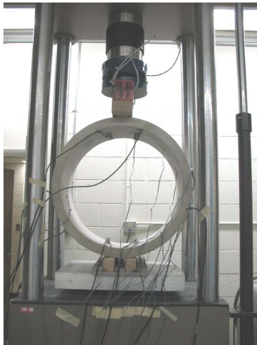
Figure B-3 The three-edge-bearing test on FRCP.
