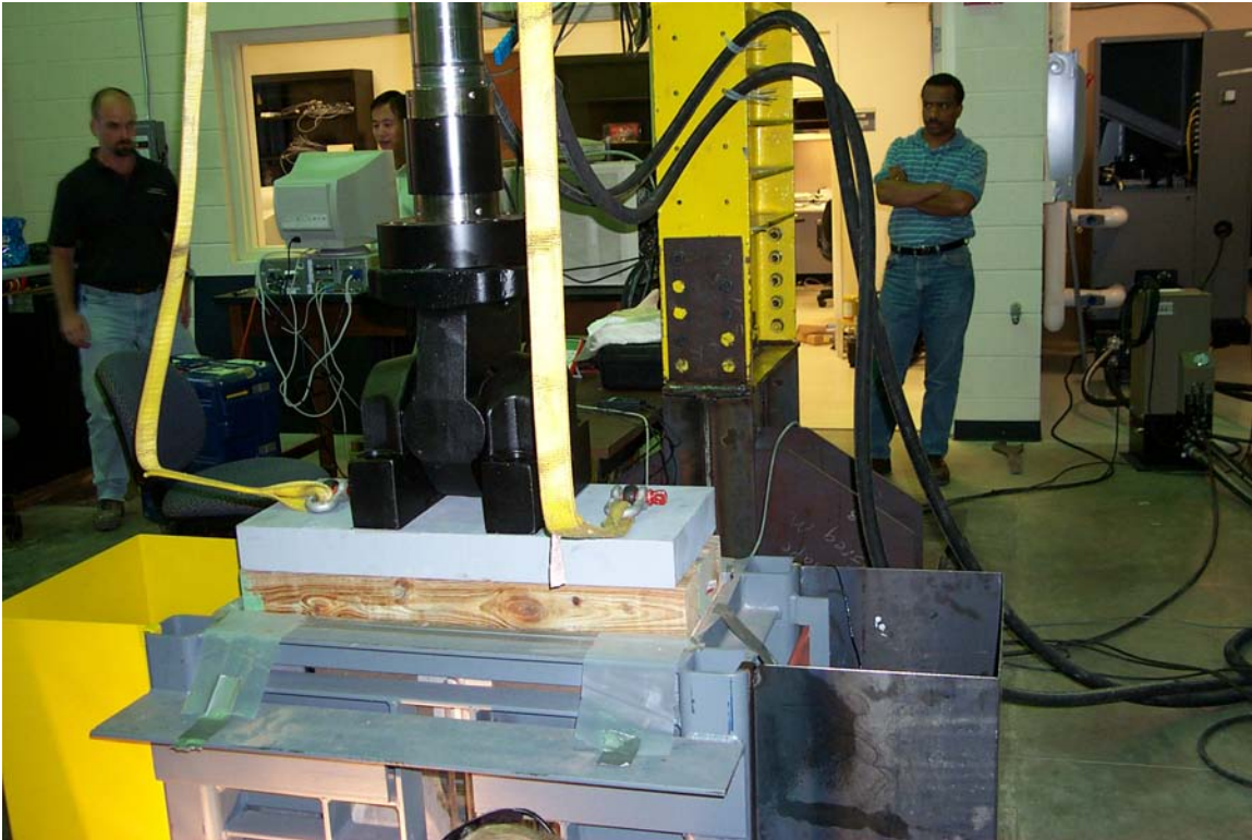
Figure A-2.8 Hardie Pipe flexible soil box testing conducted at UCF.
