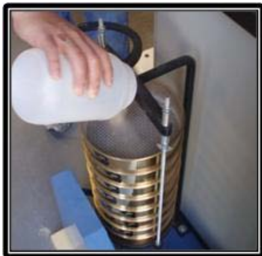
Figure 9 Apparatus for determining soil grain size analysis – ASTM D422
