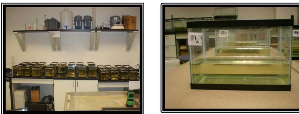
Figure 57 Test aquarium tanks for toxicity tests on PAM
