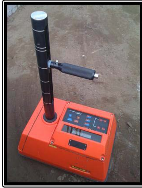
Figure 6 Apparatus for determining field moisture and density/unit weight by nuclear density gauge – ASTM D6938
