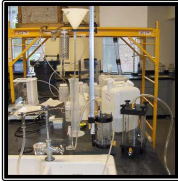
Figure 7 Apparatus for determining hydraulic conductivity of soils – ASTM D2434
