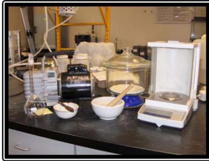
Figure 11 Apparatus for determining specific gravity of soil – ASTM D854
