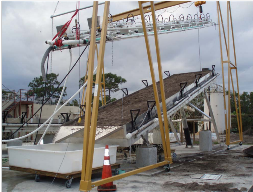
Figure 8 Configuration of Erosion Control Test Bed and Rainfall Simulator
