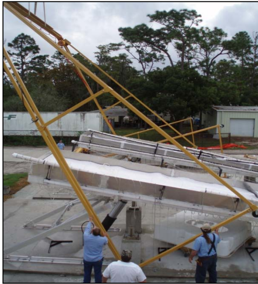
Figure 5 Installation of Gantry Crane System to Suspend Rainfall Simulator
