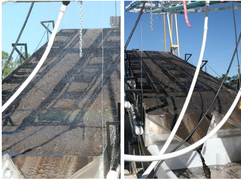
Figure 9 Example Runoff from a Rainfall Event on a Bare Soil Surface
