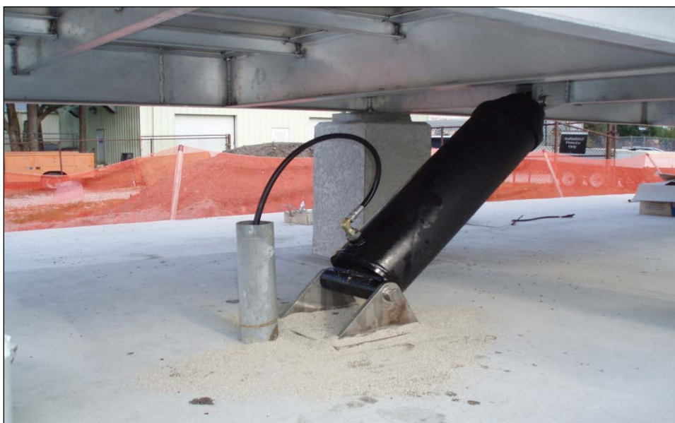
Figure 3 Hydraulic System Used to lift a Test Bed to Obtain Different Slopes
