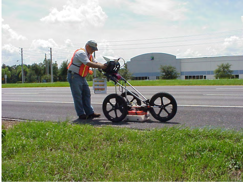
GPR Survey at Sandlake Road Test Site
