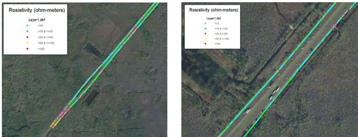
Figure 20 – Near-Surface Resistivity Along a Portion of the S.R. 400 Test Site
