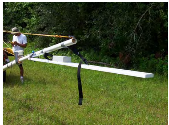
Figure 5 – Dual Antenna GPR and GEM-2 Equipment
