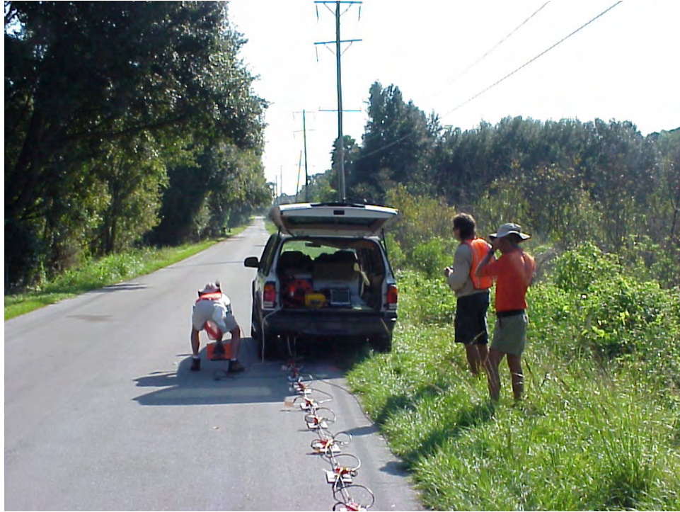
MASW Test Shot at Glen Harwell Road Test Site
