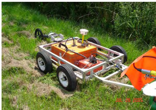
Figure 5 – Dual Antenna GPR and GEM-2 Equipment
