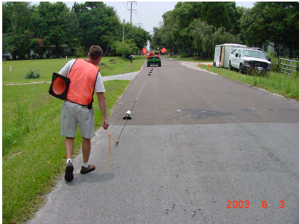
CCR Survey at Beauchamp Road Test Site
