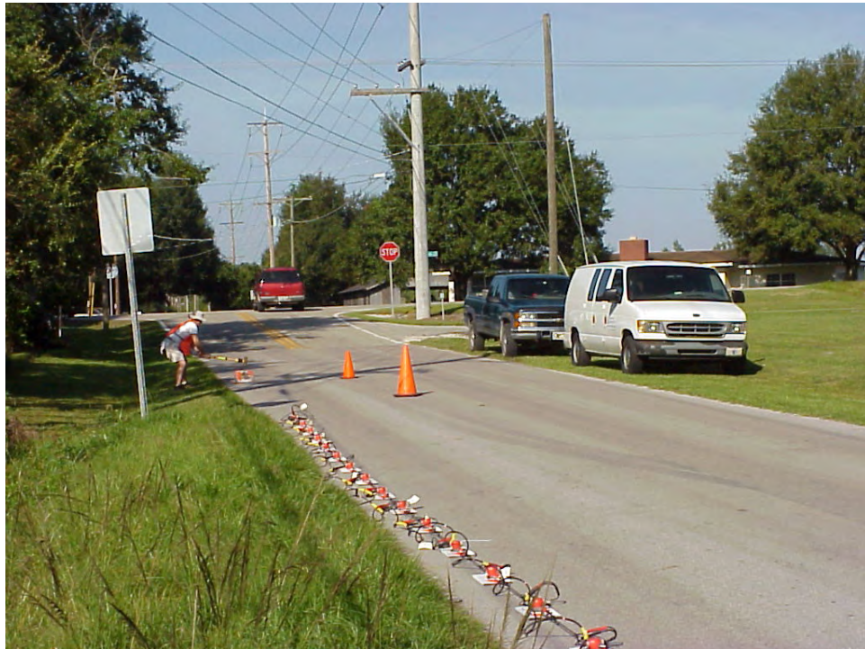
MASW Survey Shot at Glen Harwell Road Test Site
