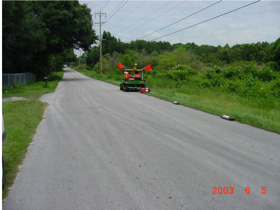
CCR / GPR Suvey at Glen Harwell Test Site
