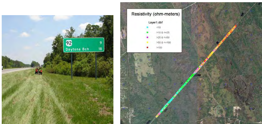
Figure 18 – S.R. 400 Validation Test Site and CCR Resistivity Overview
