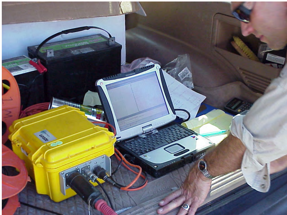
MASW Data Acquisition Set-up
