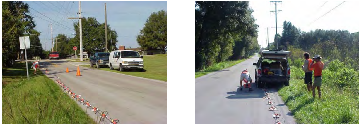
Figure 6 – Plate-Mounted Geophone Land Streamer Fabricated for MASW Testing
