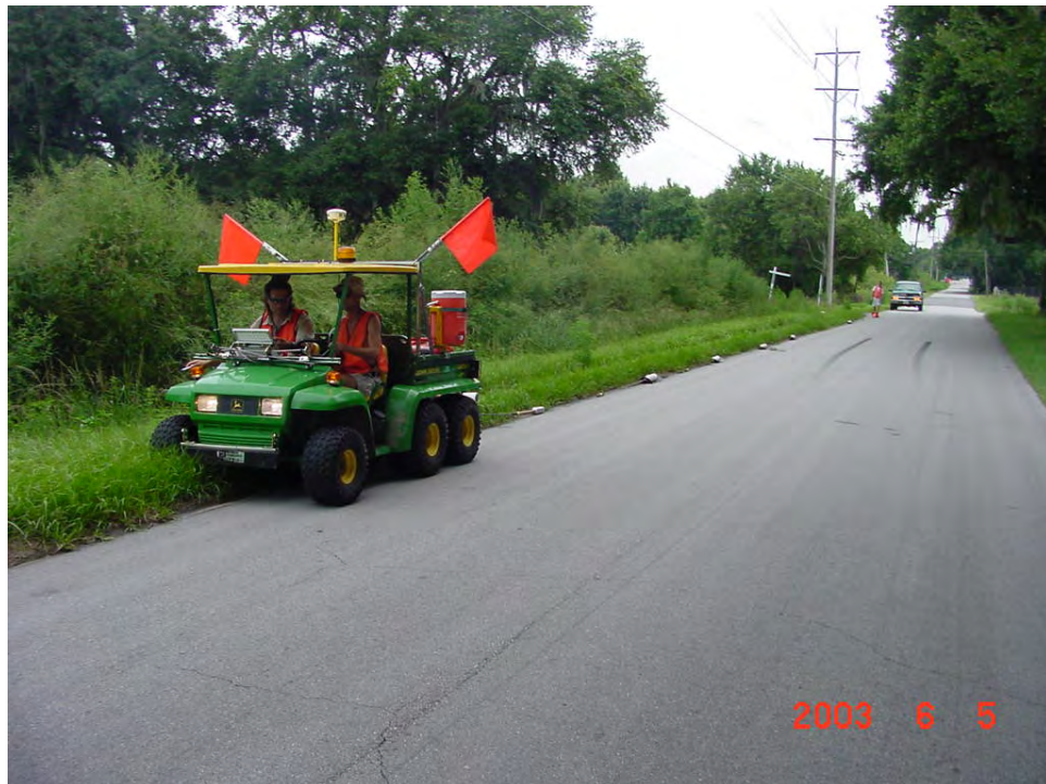
CCR / GPR Survey at Glen Harwell Road Test Site
