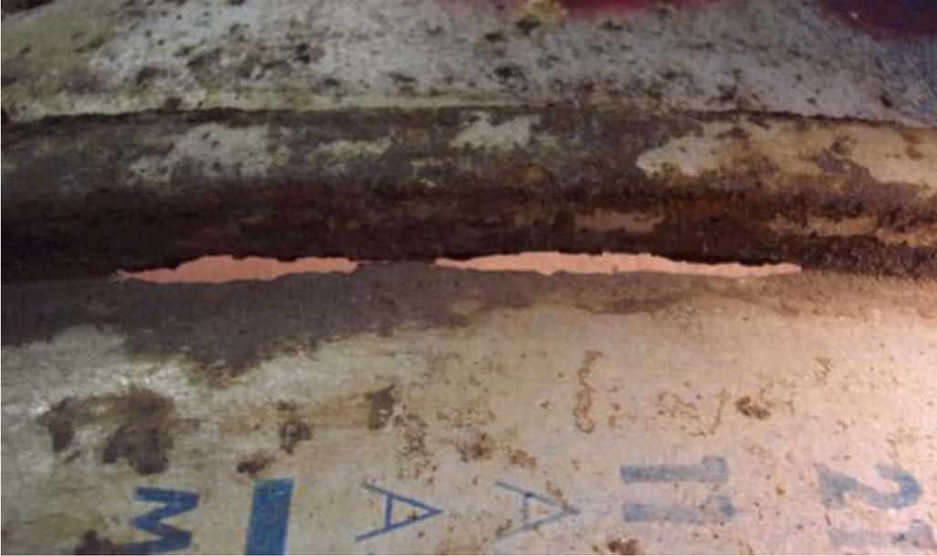
**Figure 5-4a.** Coupon #1 outer rib after cleaning.
