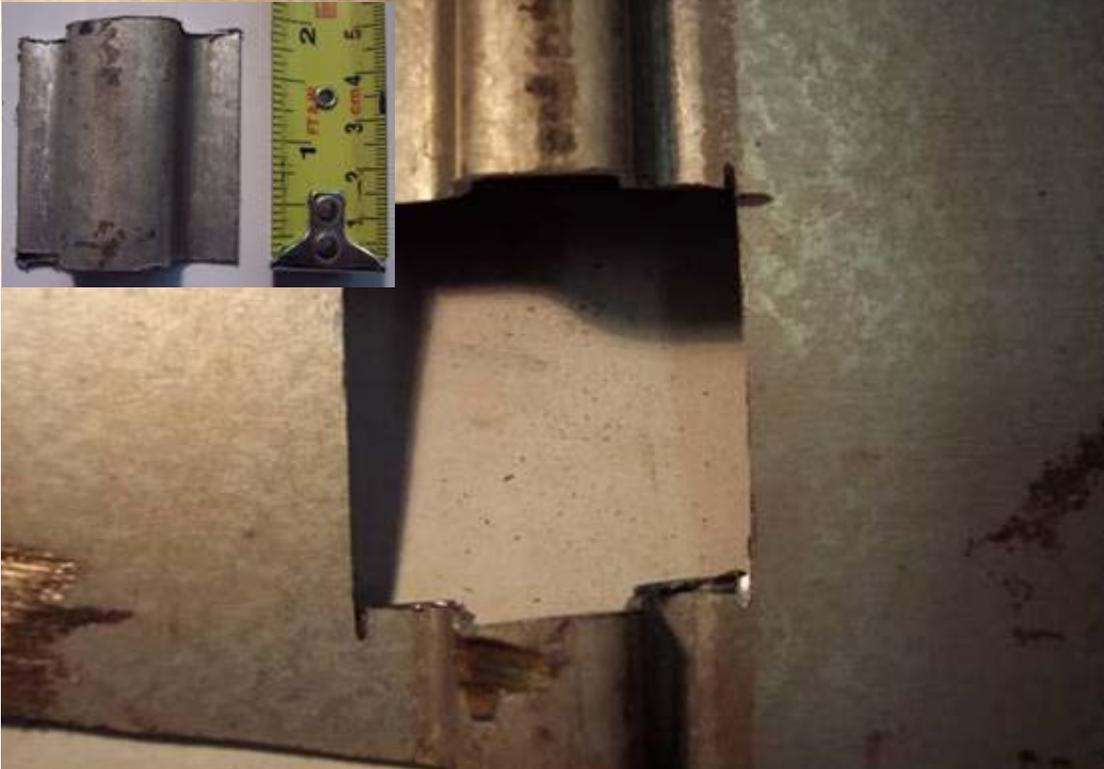
**Figure 5-7.** Spiral rib sample cut out from coupon #3 used for metallographic analysis.
