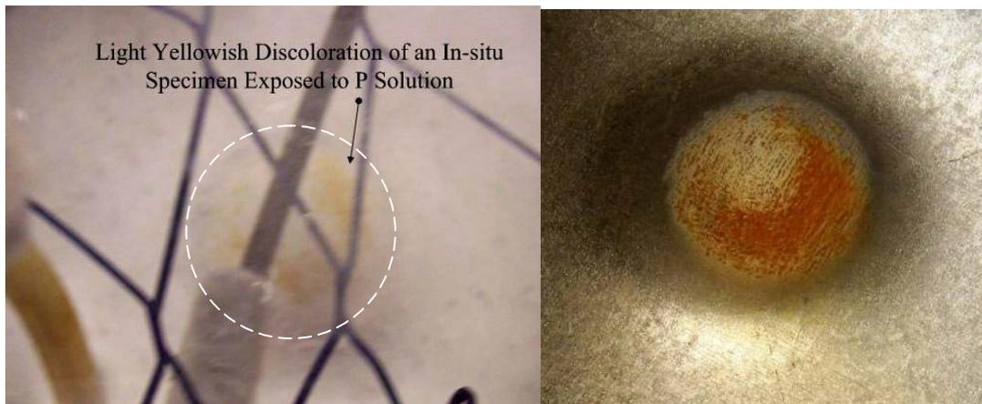
**Figure 7-6.** Light corrosion on a 2.54-cm (1-in) convex dimple immersed in solution P after 21 days of exposure (left) and severe corrosion on a 2.54-cm (1-in) convex dimple immersed in C solution after 19 days of exposure (right).
