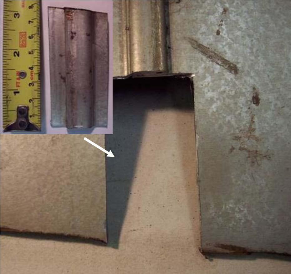
**Figure 5-8.** Lock seam sample cut out from coupon #3 used for metallographic analysis.
