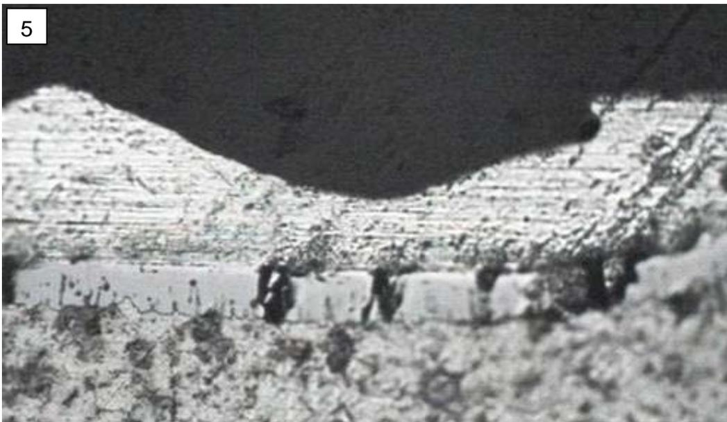
**Figure 5-9c.** Cross section for features 4 and 5. Inner layer is  $\sim 10 \mu\text{m}$  thick.
