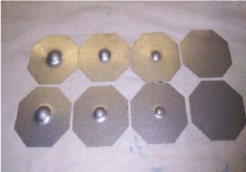
**Figure 7-3.** Duplicate specimens indented to (left to right) 2.54 cm (1 in), 1.90 cm, (3/4 in), 1.43 cm (9/16 in), and flat.
