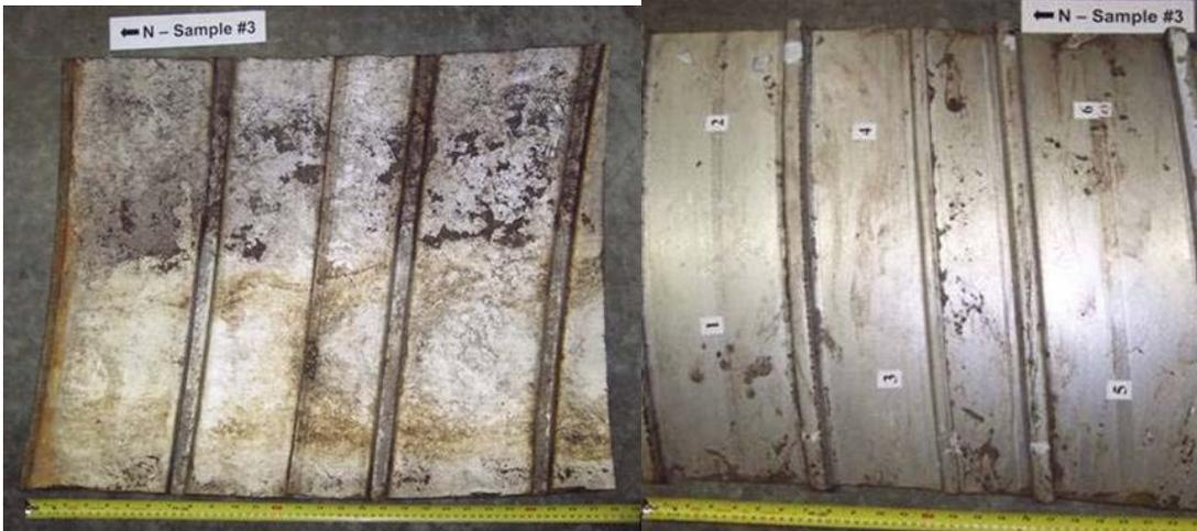
**Figure 5-3.** Coupon #3 corrosion before cleaning on water side (left) and soil side (right).
