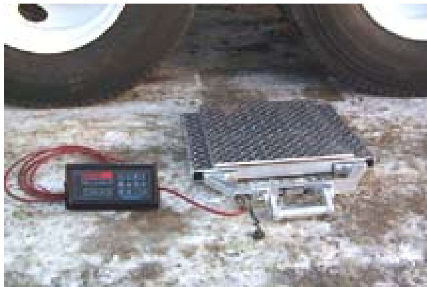
Figure 6.3. Portable wheel weigher scale.
