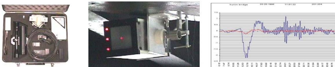
Figure 2.18. Noptel laser displacement measurement device.
