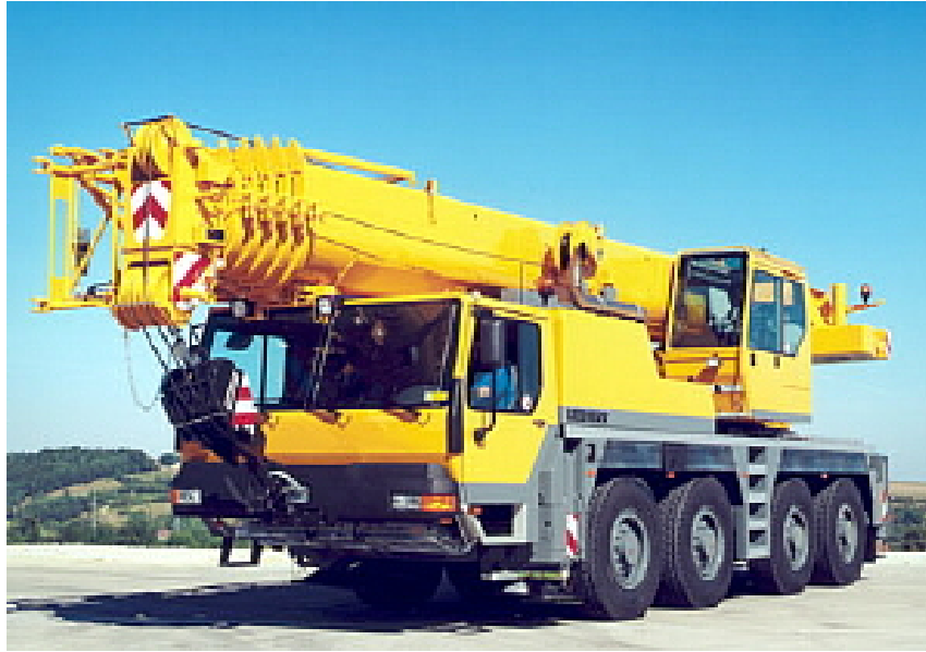
Figure 4.54. The selected crane (LTM 1080) for FE development.
