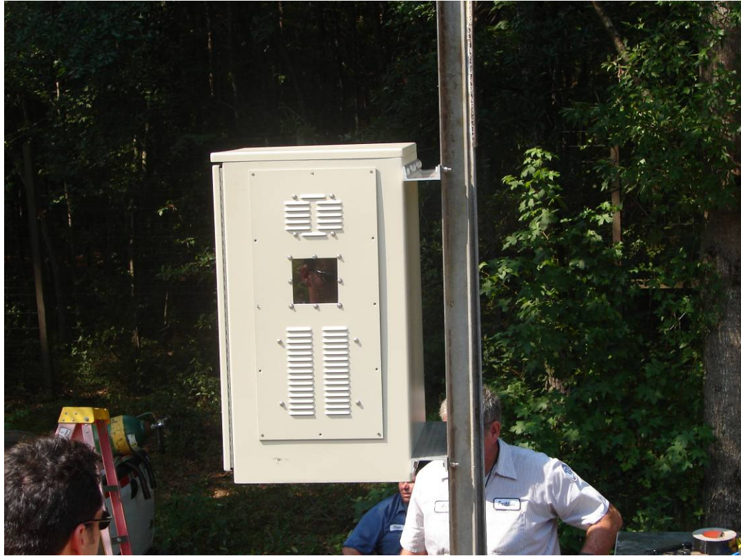
Figure 56: The UCF enclosure with window for the camera
