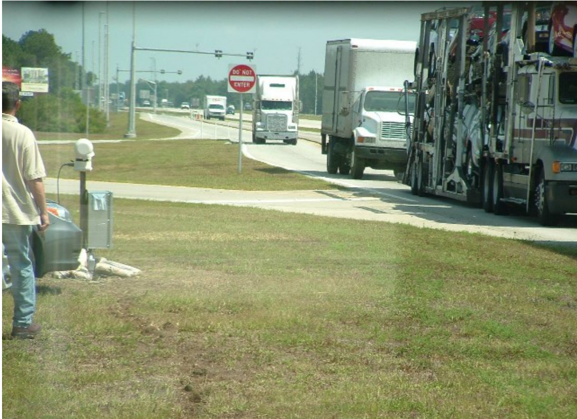
Figure 1: Camera deployment at the entrance of WIM station
