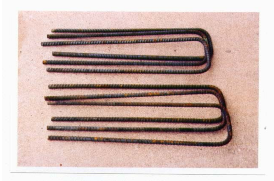
Figure A-7: Photograph of MMFX-II™ reinforcement details acquired from the job site.
