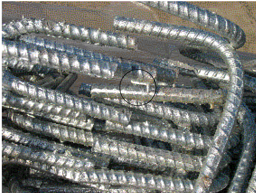
Figure E-11: Galvanized layer disbanding and icicle on reinforcing bars. Examples of disbonding are also apparent.
