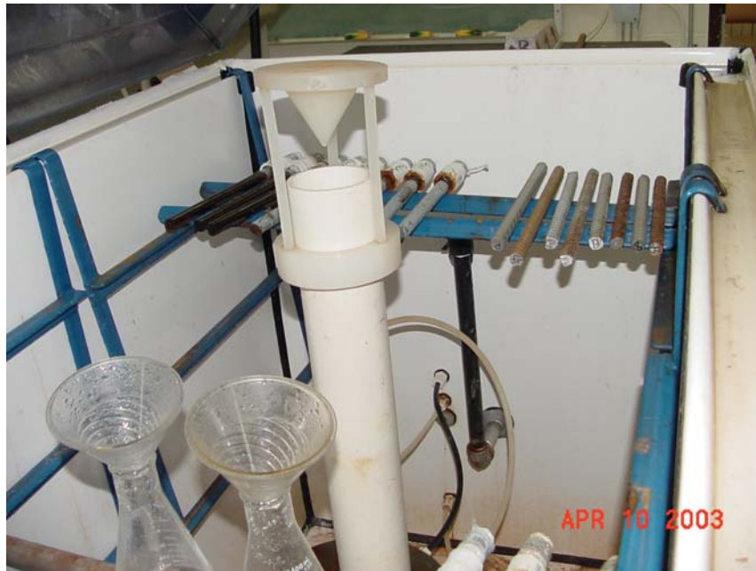
Figure B2-A1. Bars Positioned in salt fog chamber.
