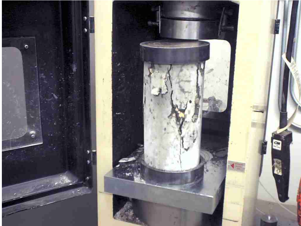
Figure 3.7: Cylinder Test in Forney Compression Machine
