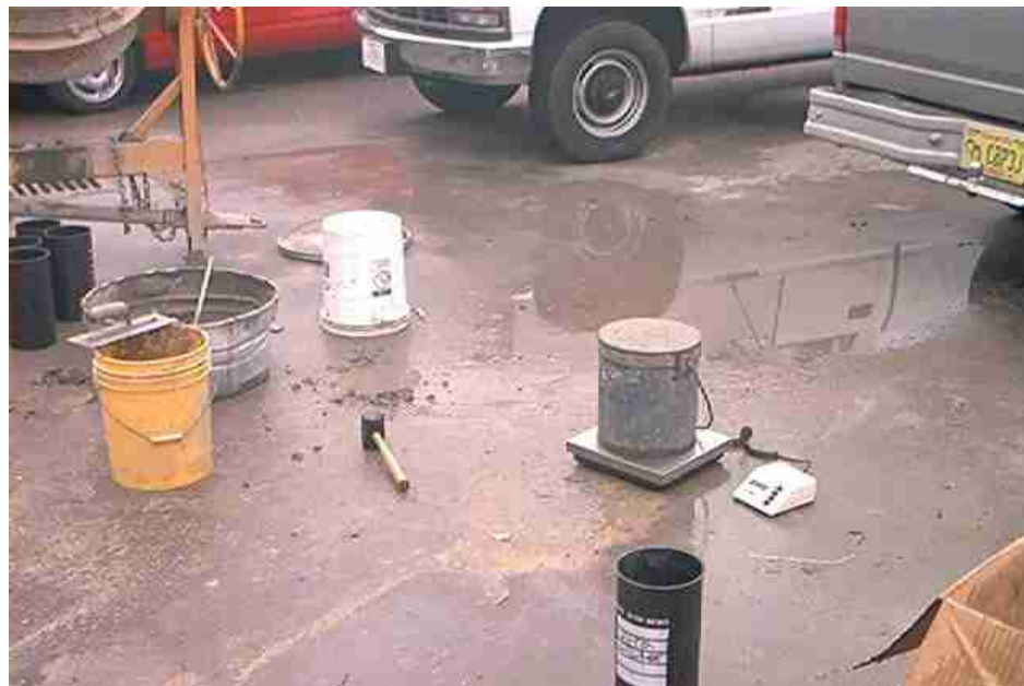
Figure 3.6: Unit Weight Test
