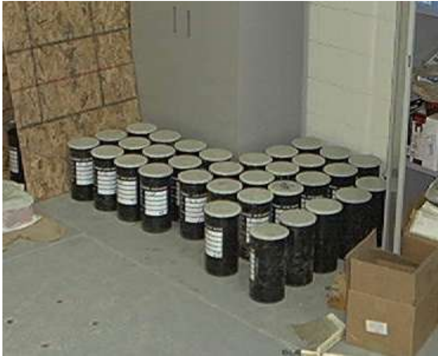
Figure 3.3: Cast Concrete in Cylinder Molds
