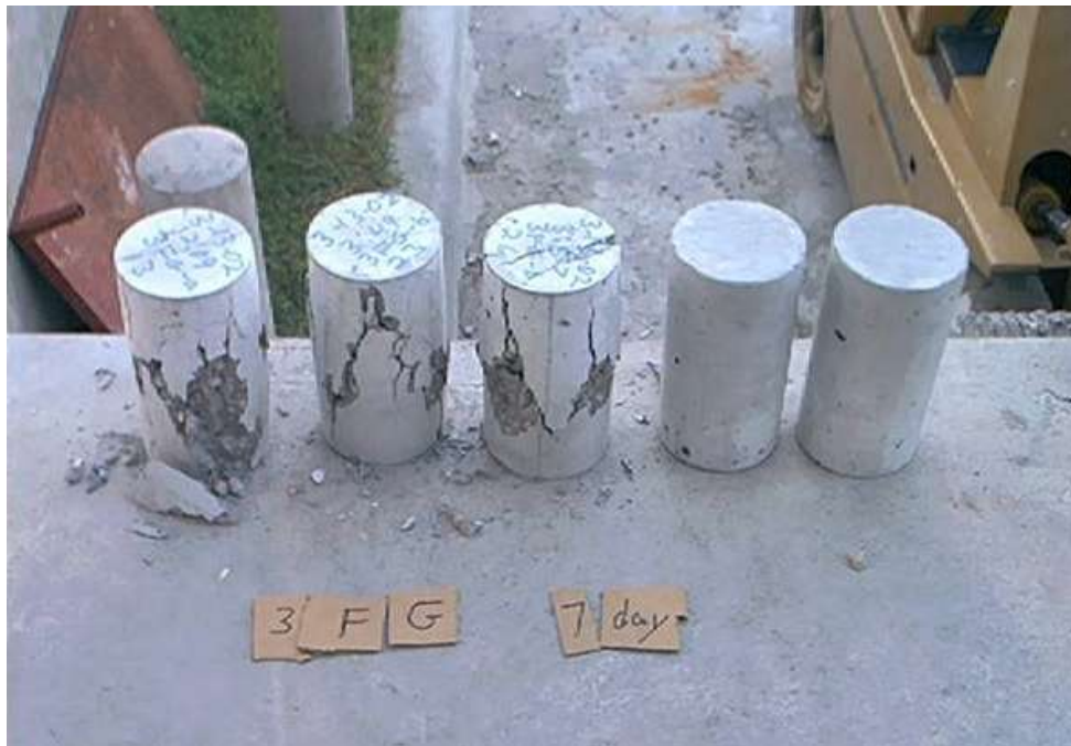
Figure 3.8: Three Cylinders from Strength Test and Two Cylinders from MOE Test
