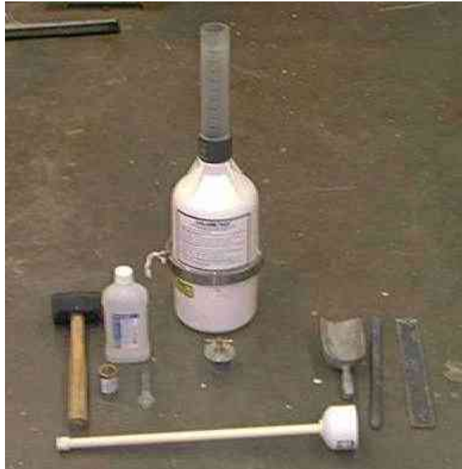
Figure 3.5: Volumetric Air Content Test
