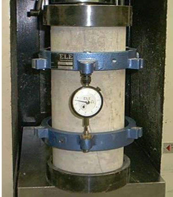
Figure 3.9: Compressometer Attached to MOE Test Sample
