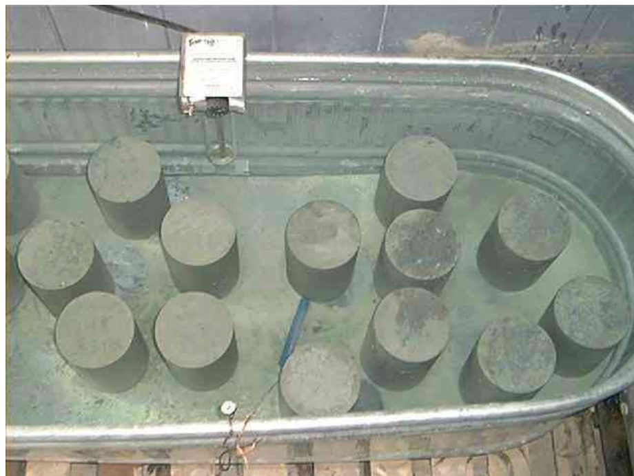
Figure 3.4: Curing Tank with Heater and Thermometer
