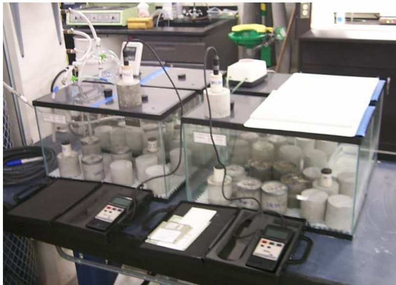
Figure 21: Photograph of constant RH chambers with specimens, embedded RH probes(2), and meters(2).
