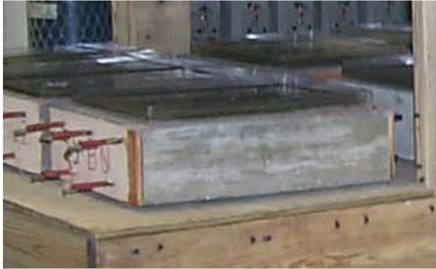
Figure 6: Photograph of an individual concrete slab specimen from the previous admixture project.
