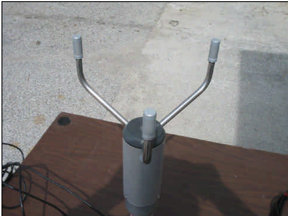
ANEMOMETER Coastal Environmental Systems (Part Number: S5777)
