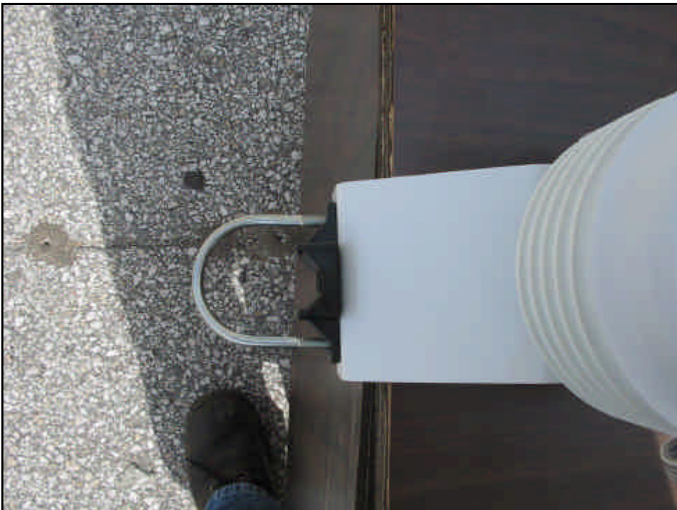
ASPIRATOR Coastal Environmental Systems (Part Number: S1276Z) (Temperature and Relative Humidity Sensors)
