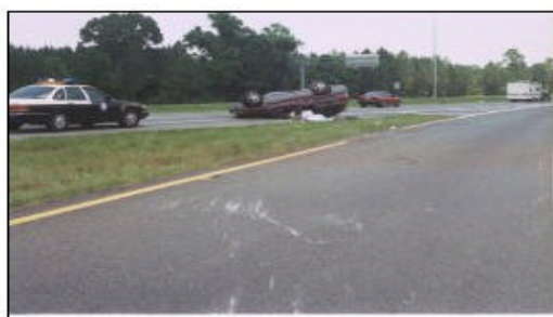
Photo 3: Scratches on pavement due to rollover
