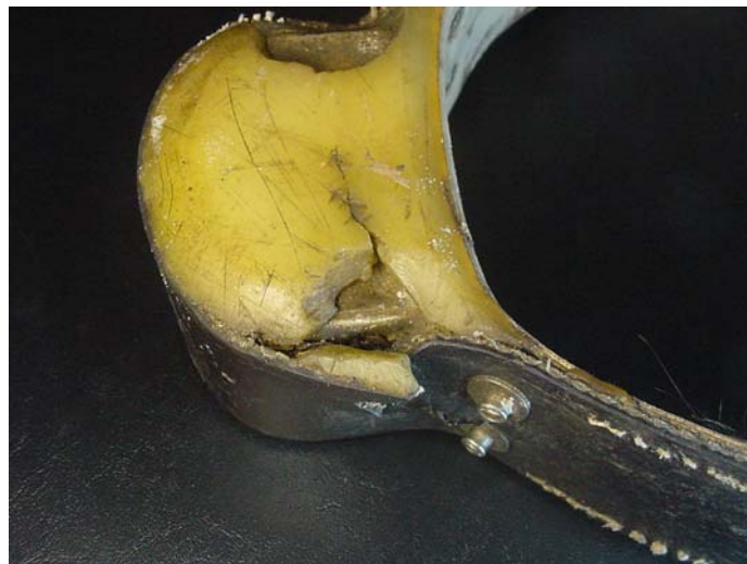
Radio collar of male bear number 8 with damage resulting from an aggressive encounter with another bear.
