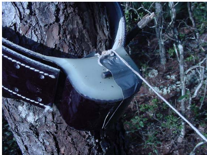
Alarm collars were rigged to activate when a string fastened to the anchor cable was tugged sufficiently to pull the deactivating magnet from the collar.
