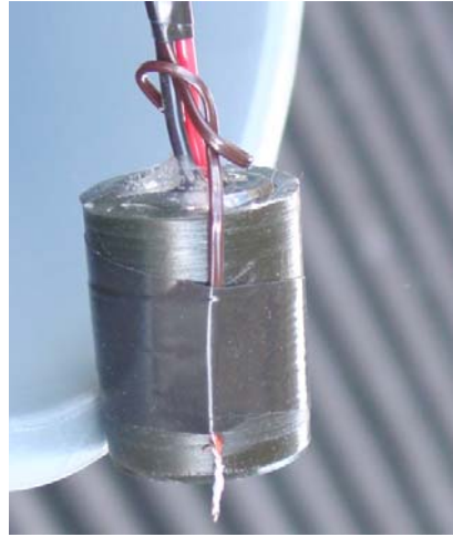
Figure 3.8a: S-type and NS-type Sensors Tied Together to Measure Maturity at the Same Point
