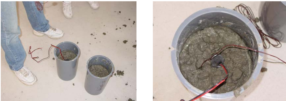
Figure 3.5: Installation of Maturity Sensors in the Trial Test Cylinders
