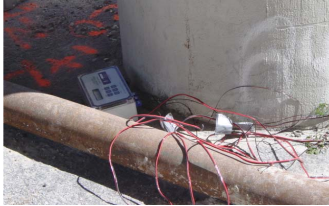
Figure 3.10: Data Recording from Non-Sacrificial Sensors (Humboldt™ System)
