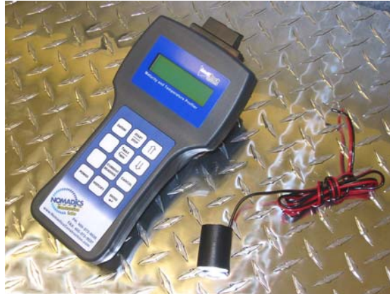
Figure 3.2: The IntelliRock TM Handheld Reader and a Logger
