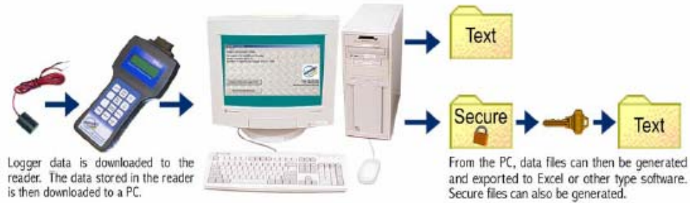
Figure 3.3: Data Transfer Process from the Reader to the Computer in the IntelliRock™ System (Goodrum et al., 2004)
