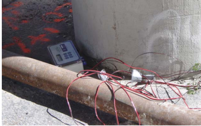
Figure 3.10: Data Recording from Non-Sacrificial Sensors (Humboldt™ System)
