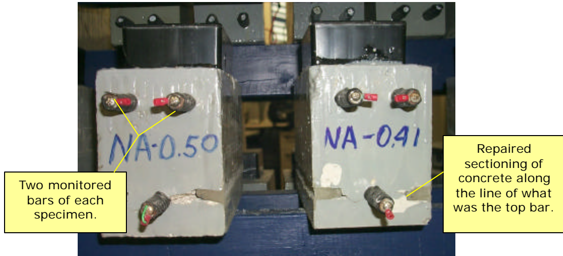
Figure 27: Photograph of two repaired and inverted specimens under test.
