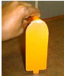
FIGURE 4-1. The Wisconsin Device for Maintaining a Uniform Installation Depth
