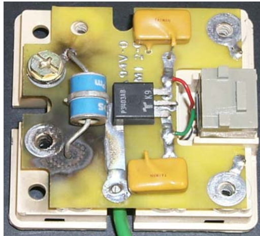
Figure 9. Burned Pads for EDCO
