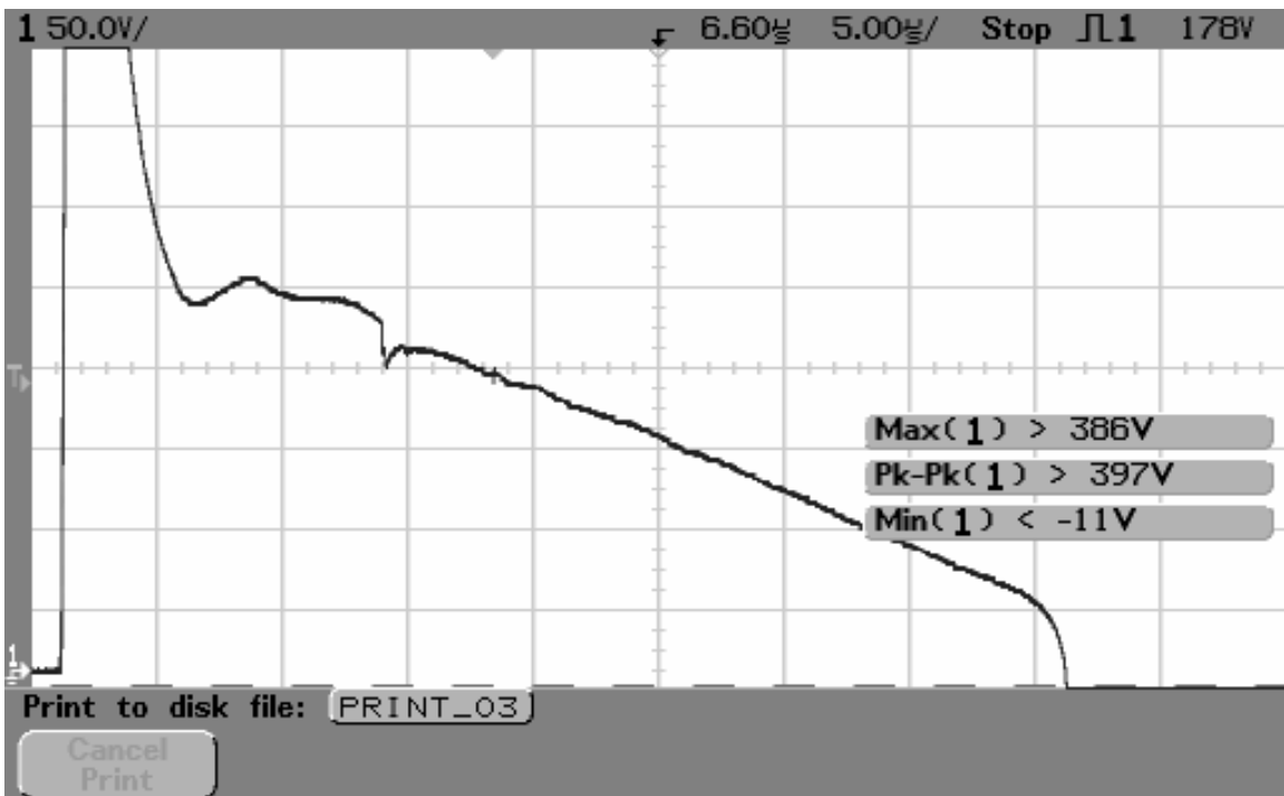
Figure A.9. S-TC-2 Surge Suppressor Output Voltage
