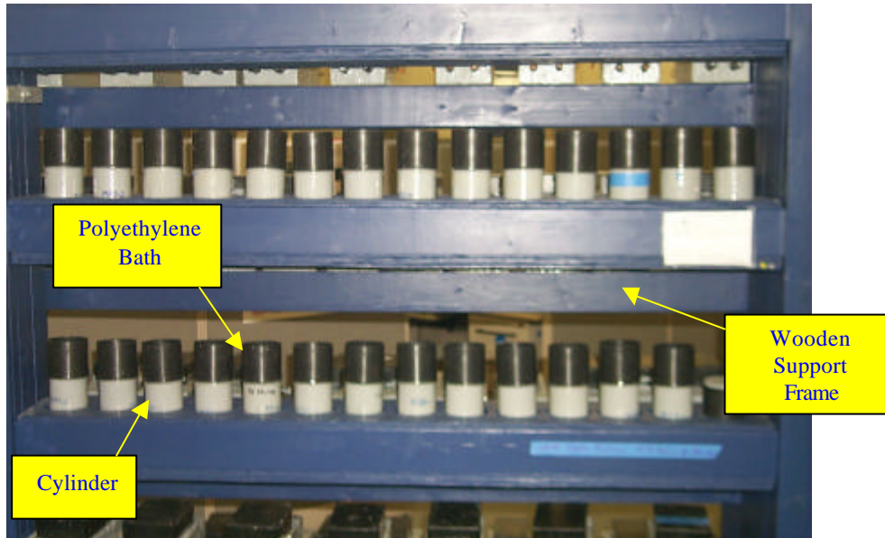
Figure 7: Photograph of mortar specimens under exposure testing.
