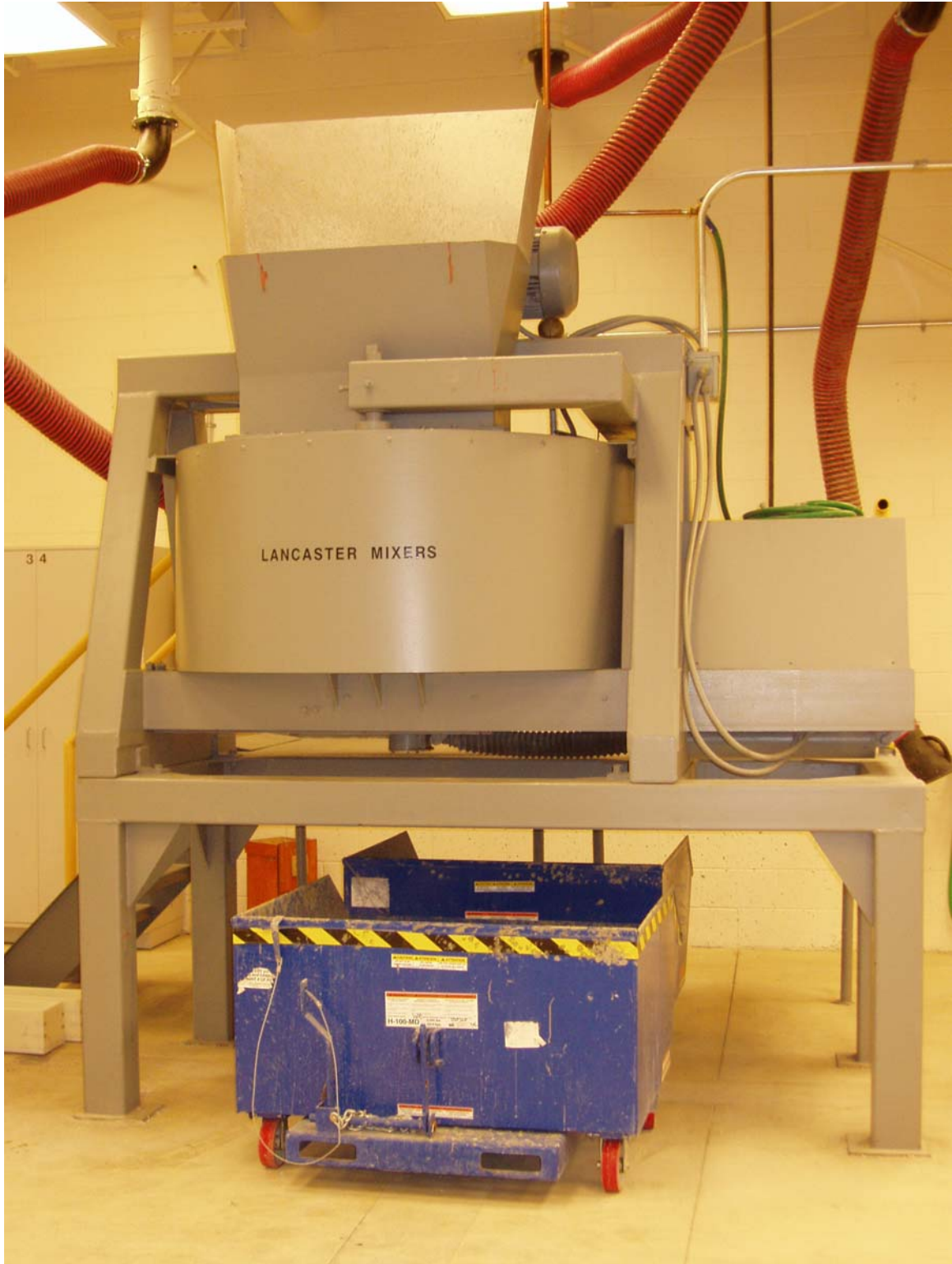
Figure 4-4. Concrete mixer used in this study
