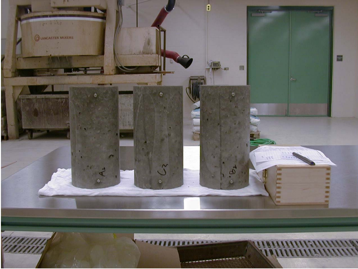
Figure 4-7. Concrete cylinders with gauge point installed on them the cylinders were brought out of the moist room. The shrinkage test was run under the conditions of the temperature of 73 °F and 75% relative humidity. The shrinkage strain was taken as the average of the nine readings from the three replicate cylinders, and can be expressed as follows:
