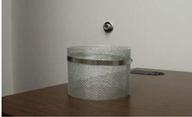
Figure 7-1. 1/8" Mesh Used for Containing the Specimen.
