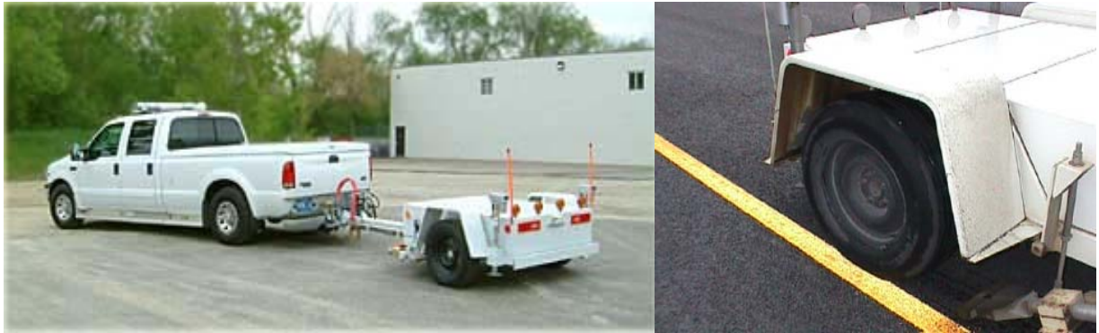
Figure 8-1. Friction Unit (Left) and Locked Wheel (Right).
