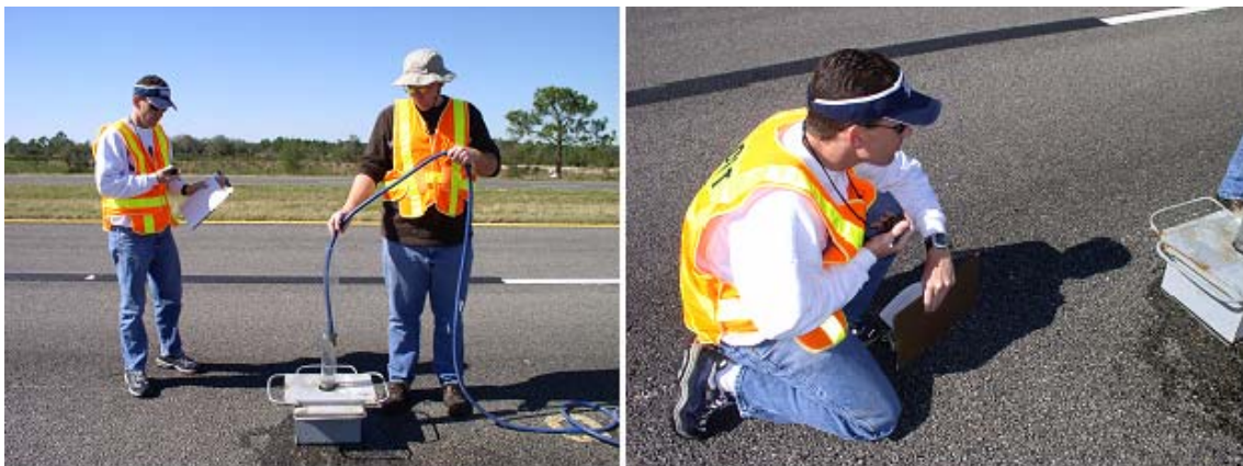
Figure 8-10. Timer Recording in Field Permeability Test.
