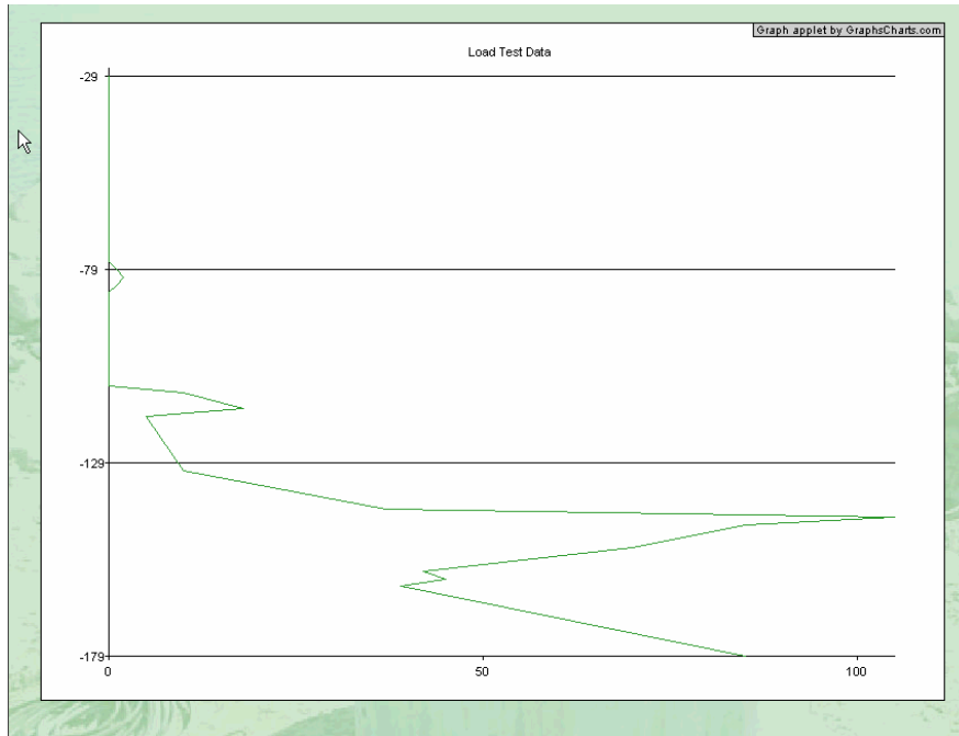
Figure 3-11 Plot of blow count vs. elevation.
