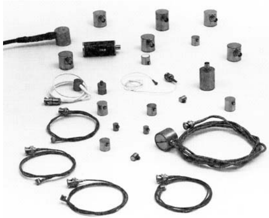
Figure 2.48: Various acoustic emission sensors. (Miller 1985)
