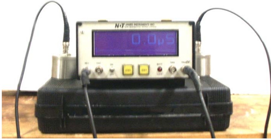
Figure 2.14: A portable ultrasonic testing device used at the University of Florida.
