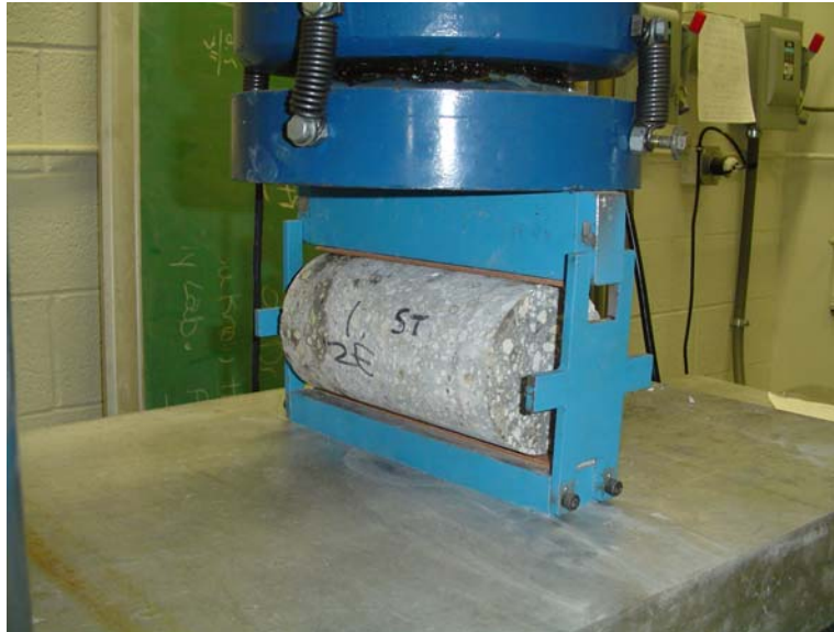
Figure 4.14: A concrete core subjected to a splitting tensile load.
