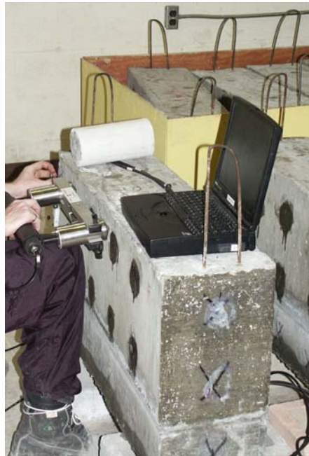
Figure 4.3: Impact-echo testing of exposure blocks.
