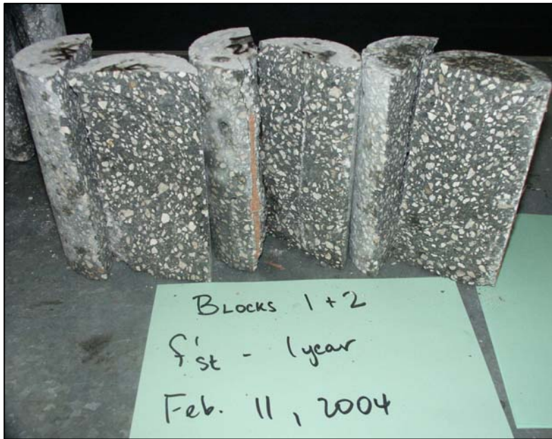
Figure 4.17: Photograph of cores failed under a splitting tensile load.
