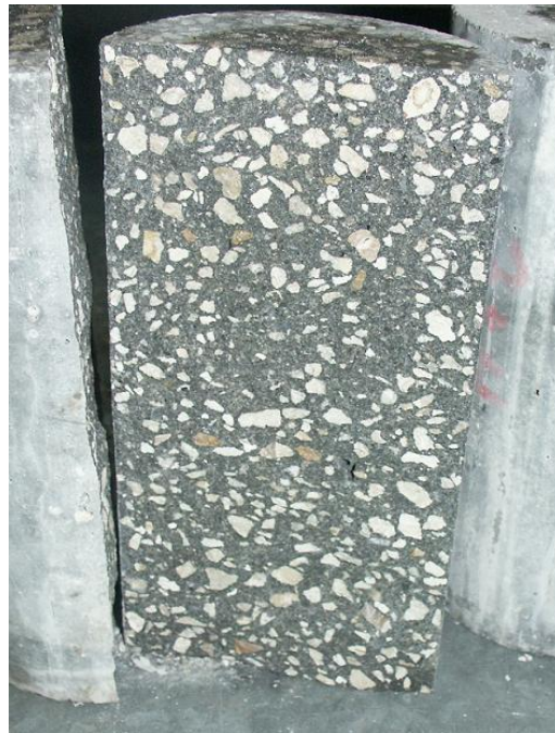
Figure 4.18: Close-up photograph of a cylinder failed under a splitting tensile load.
