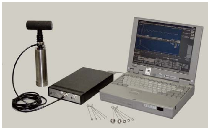
Figure 2.27: View of a typical impact-echo equipment system.
