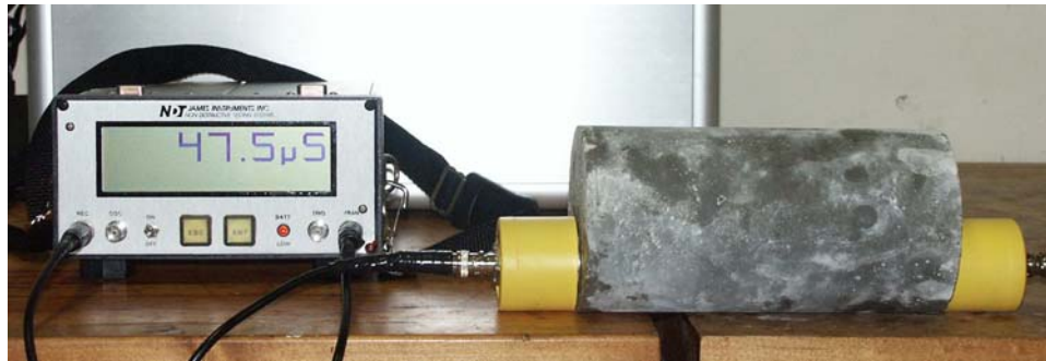
Figure 2.17: Typical ultrasonic pulse velocity test procedure.
