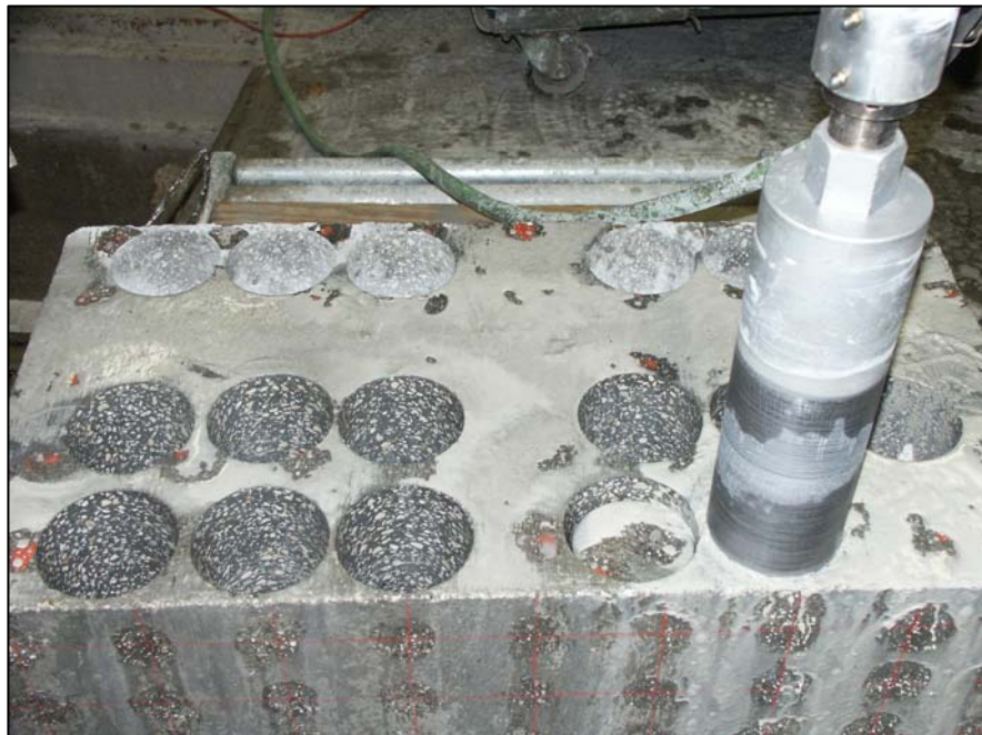
Figure 4.10: Coring technique for destructive testing of exposure blocks.
