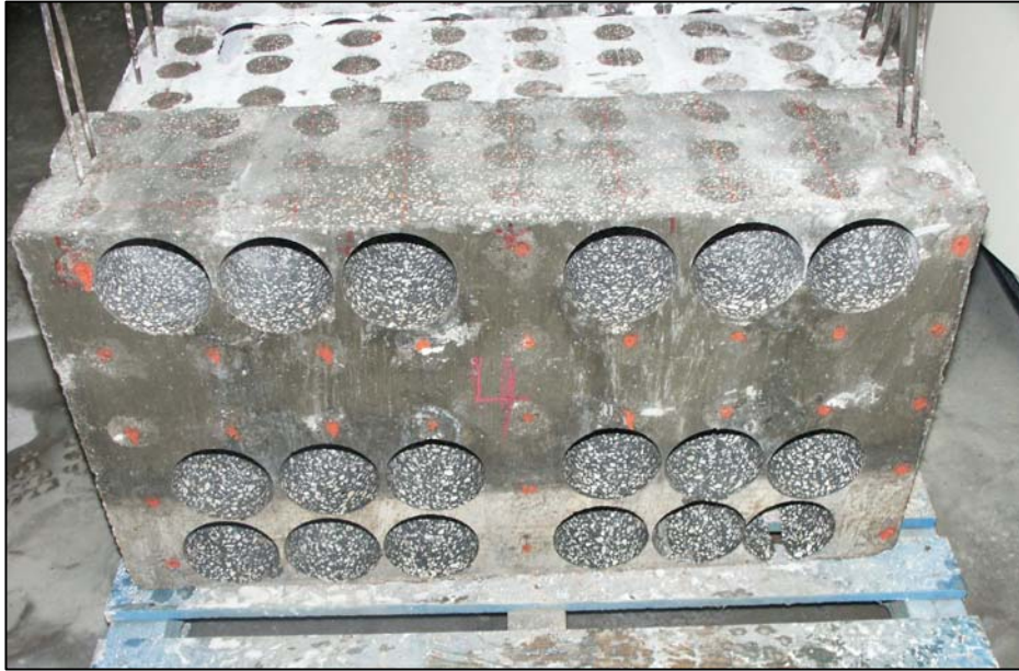
Figure 4.11: Fully cored block.
