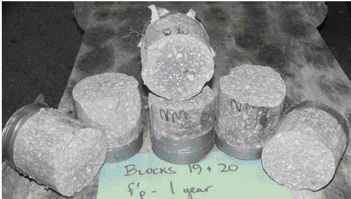
Figure 4.25: Pressure tension cores from bottom of block (sulfate solution).
