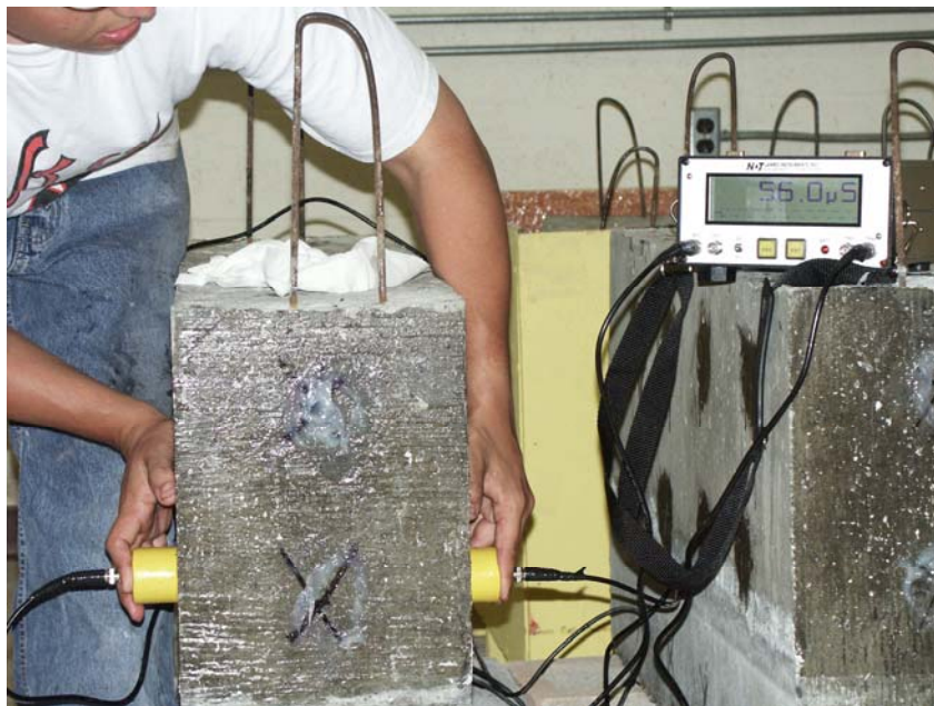
Figure 4.2: Ultrasonic pulse velocity testing of exposure blocks.
