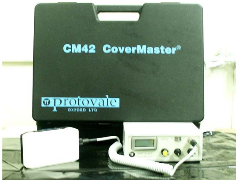
Figure 2.59: Covermeter used by the Civil Engineering Dept at the University of Florida
