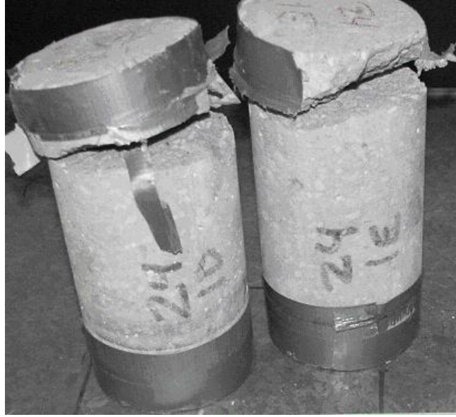
Figure 4.23: Pressure tension cores from top of block (sulfate solution).
