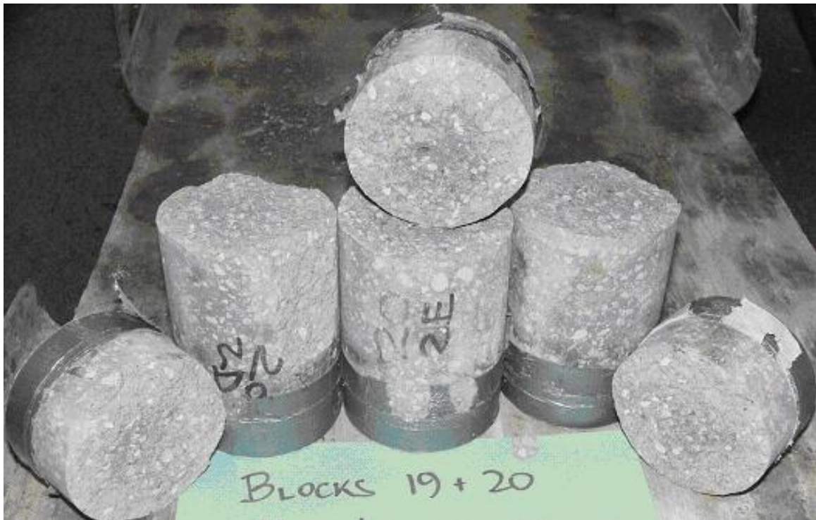
Figure 4.24: Pressure tension cores from immersion line (sulfate solution).
