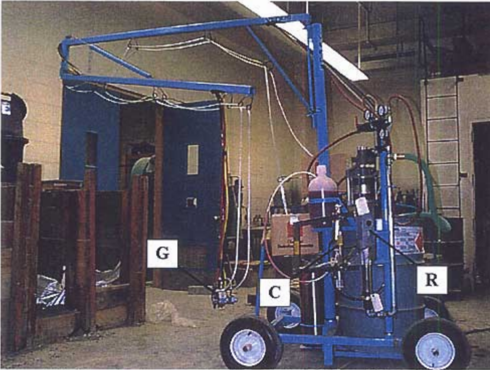
Figure 3-9: Spray Equipment: Gun (G), Catalyst (C), and Resin (R)
