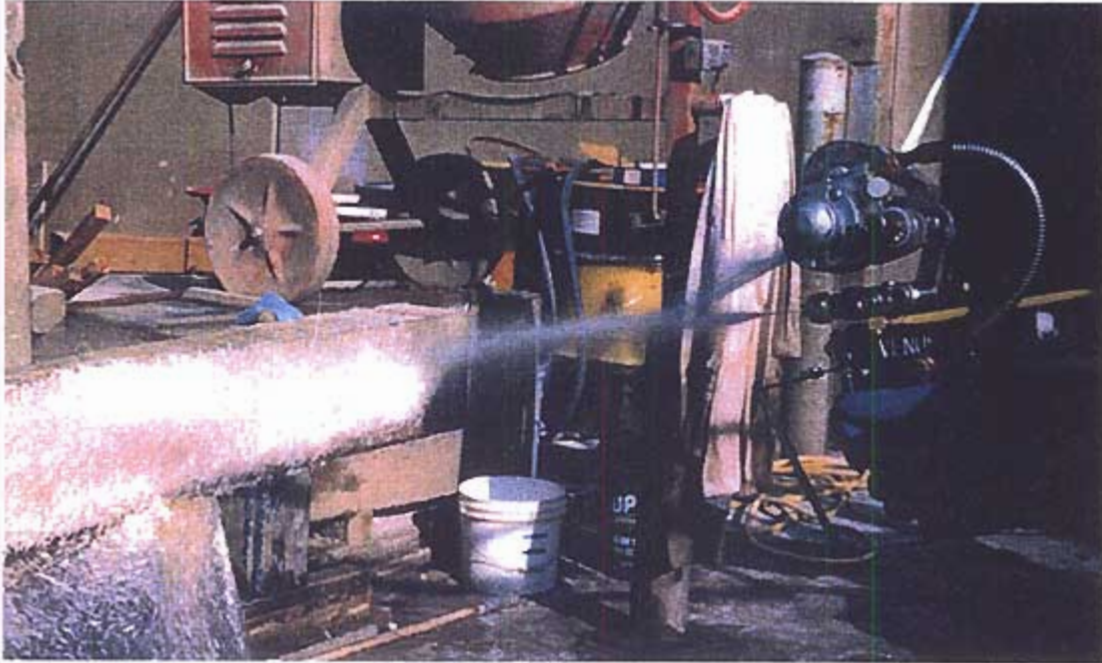
Figure 3-11: Spray Technique Procedure Showing How the Glass Fibers, Resin, and Catalyst for Resin are Combined in Mid-Air
