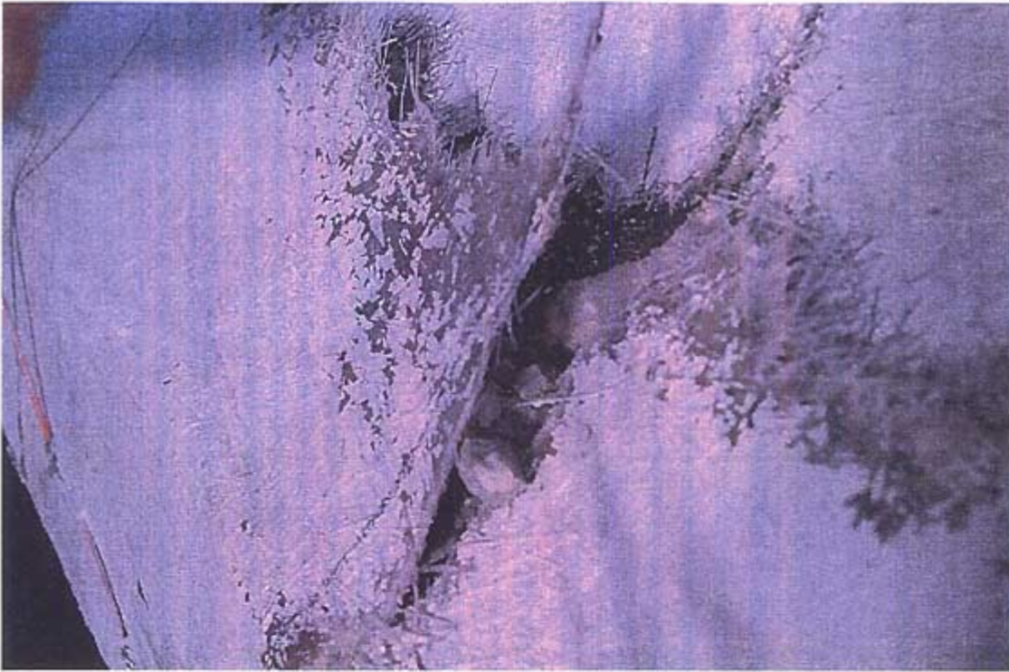
Figure 4-37: Test Specimen 5 at Failure Showing Rupture of FRP at Midspan on Tensile Face of Girder
