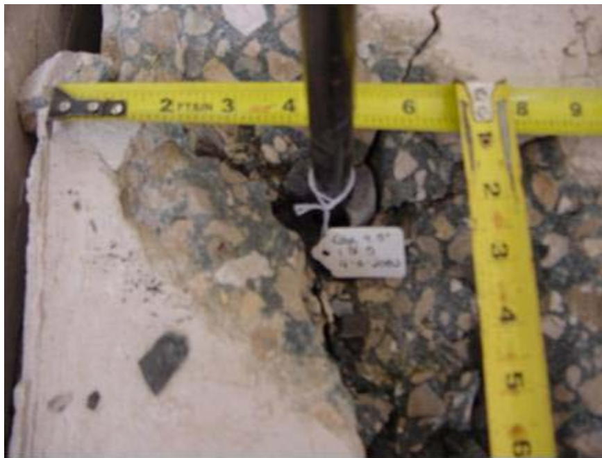
Figure E-6 Typical grout/concrete bond failure of single core-drilled anchor installed 4.5 inches from one edge with grout plug and diagonal cracking of surrounding concrete
