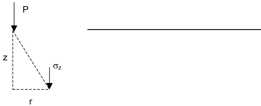
Figure 2-3. Boussinesq point load
