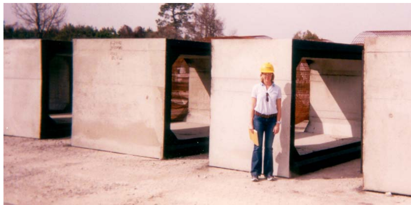
Figure 3.10: Series of 10' x 5' Precast Box Culvert Sections
