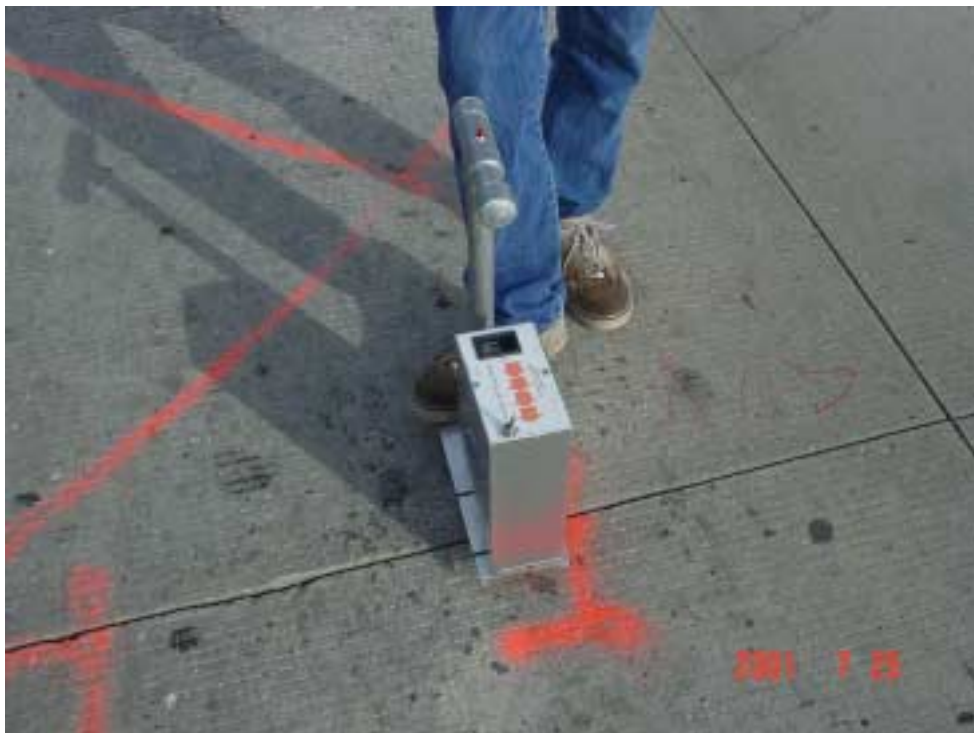
Figure 3.2 Measuring Faulting Across a Joint
