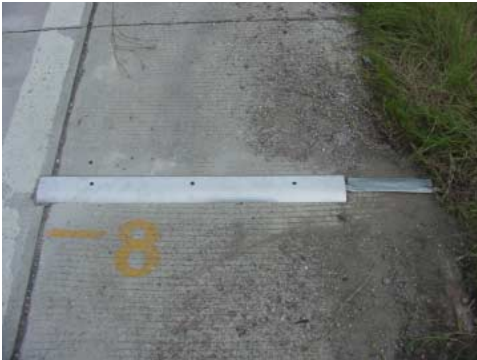
Figure 3.26 Protection of Installed Thermocouples
