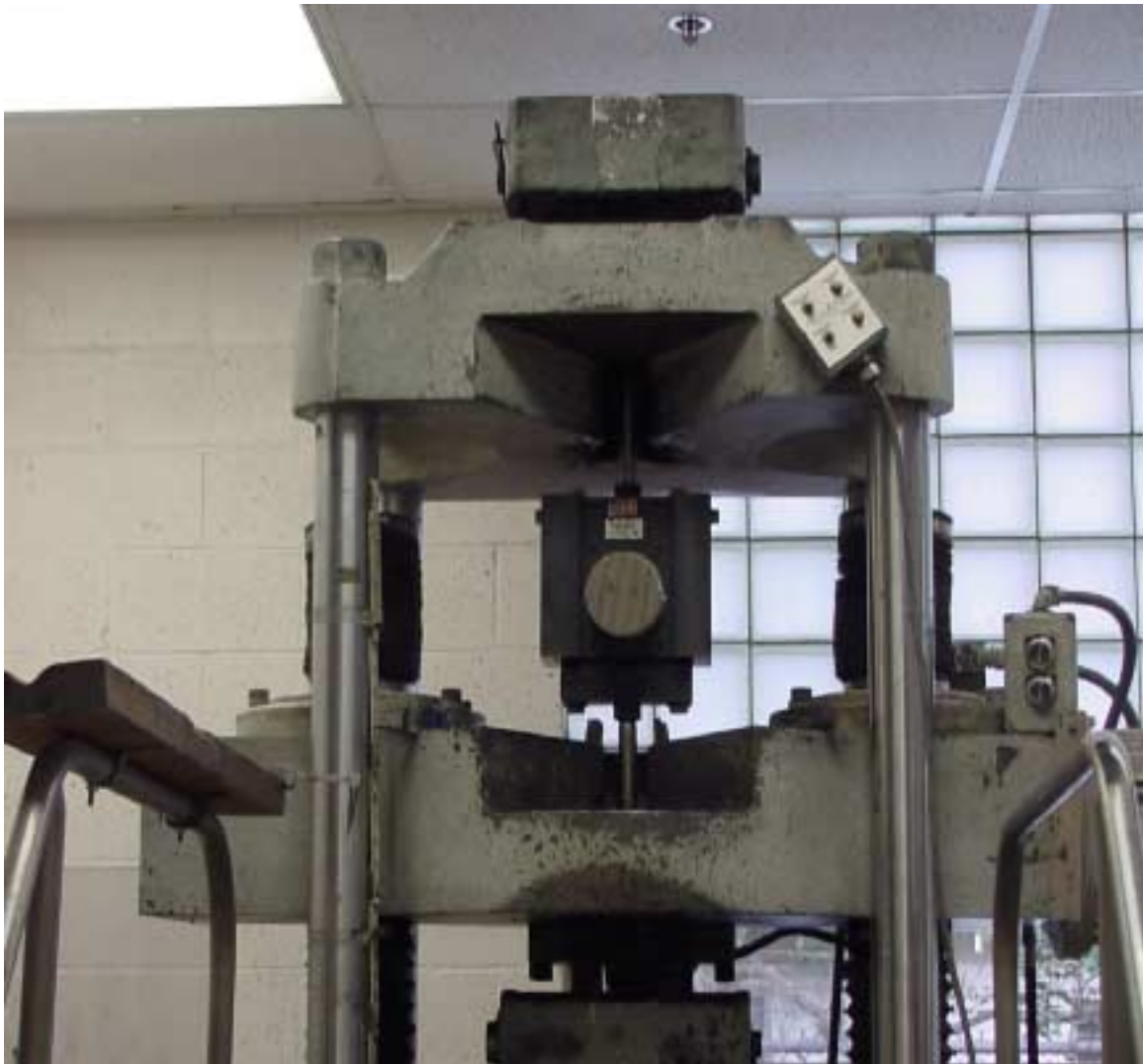
Figure 4.1 Interface Shear Strength Test Setup
