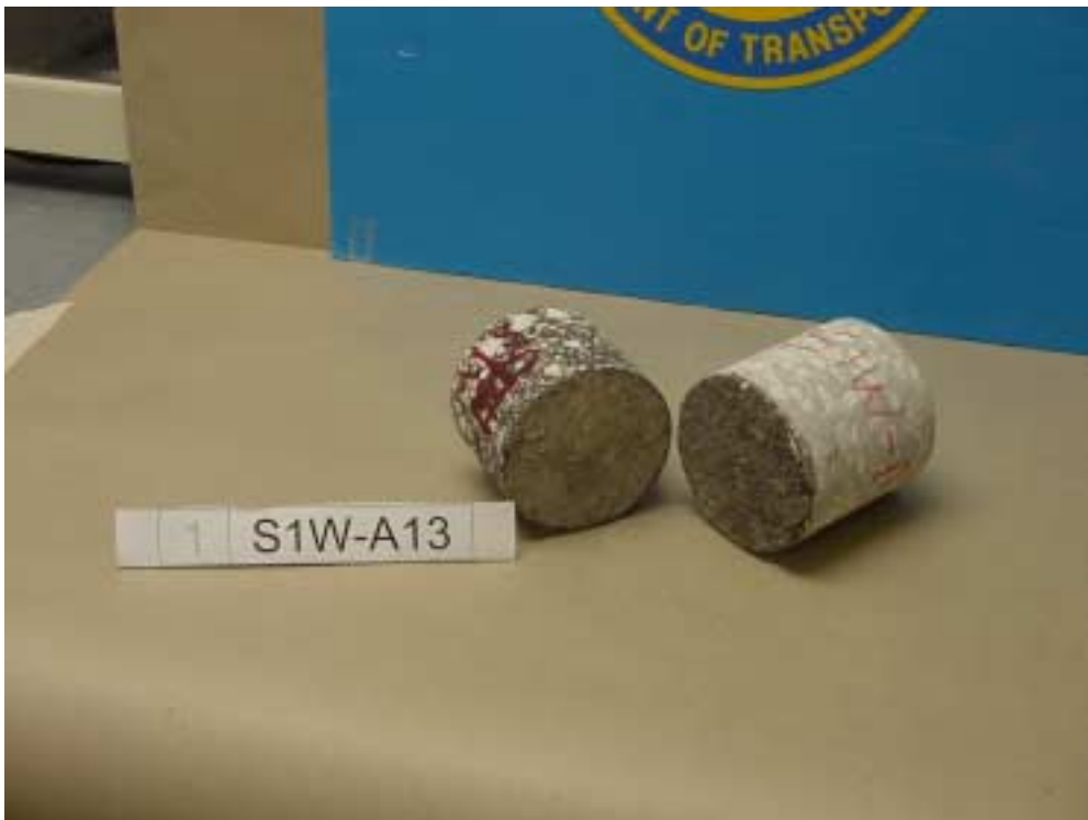
Figure 4.3 A Typical Core After Test
