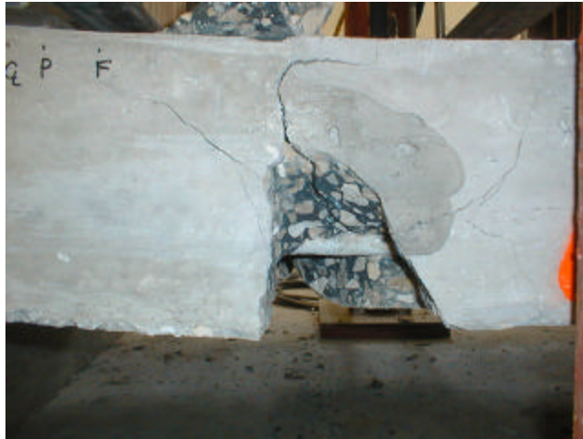
Figure 4.3 – Edge failure of Specimen B
