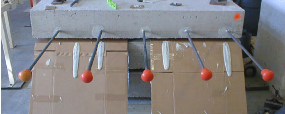
Figure 3.8 – Installed splice bars
