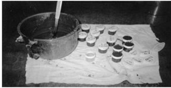
Figure. 4.1 Paste samples cast in one-ounce polypropylene screw cap jars.
