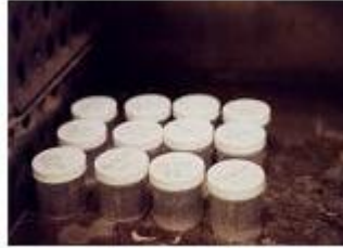
Figure 4.3 Samples cured in four-ounce polypropylene jars after demolding
