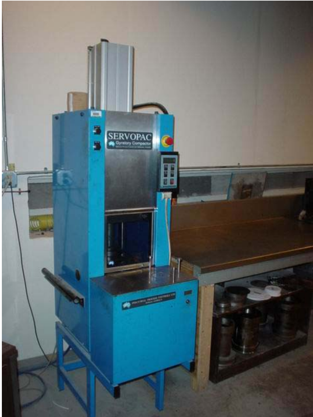
Figure 3-8. Servopac Superpave gyratory compactor
