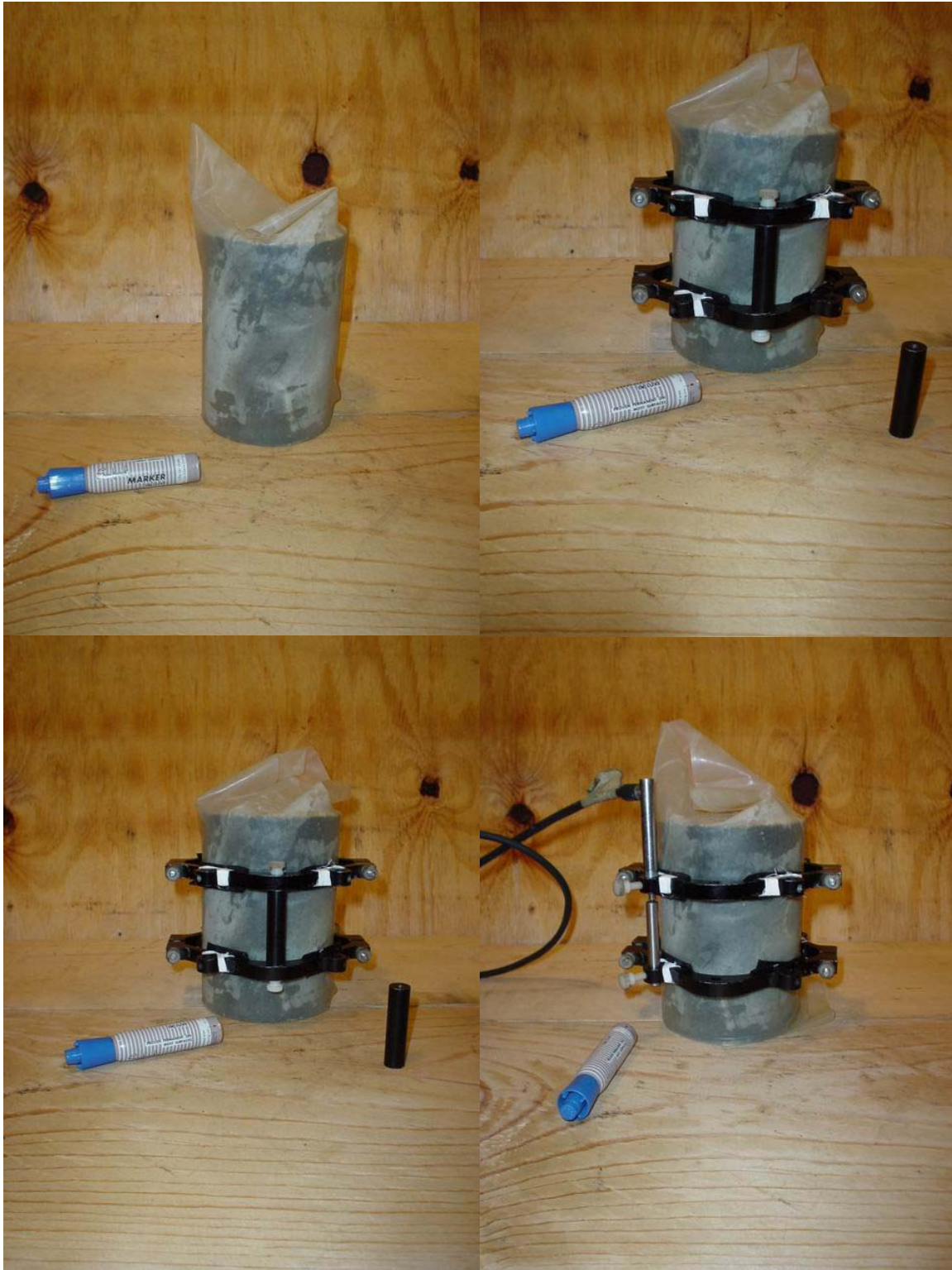
Figure 4-7. Preparation of a sample complex modulus test
