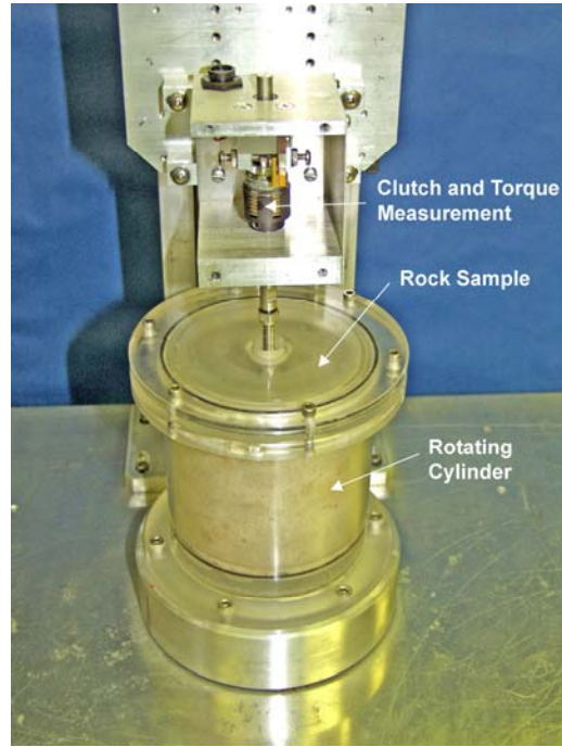
Figure I - 2. Photograph of the RETA, Viewed from Above.
