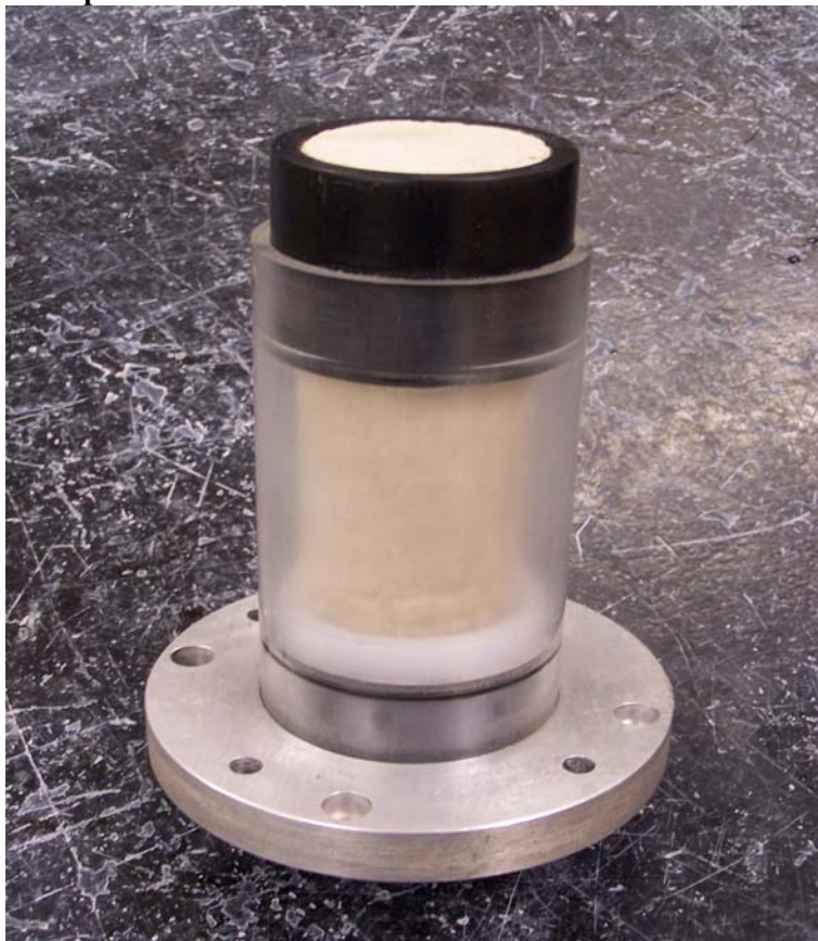
Figure IID - 9. Assembled Rock Core Test Cylinder Containing a Rock Sample.
