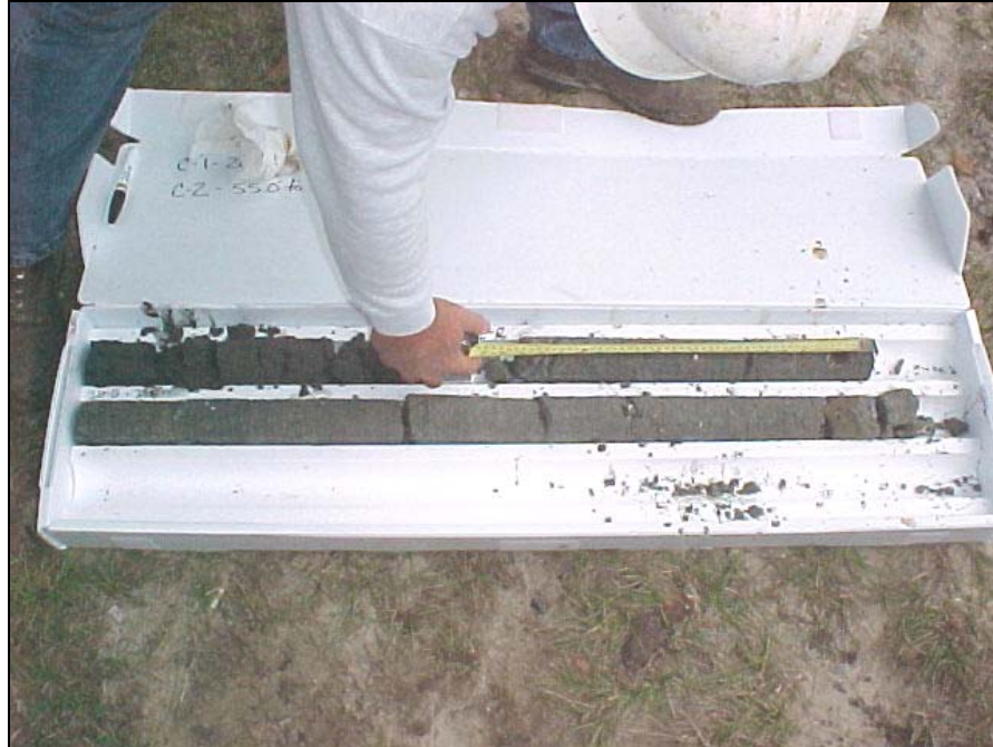
Figure 4.10: West Bay Bridge Samples Obtained from Borehole
