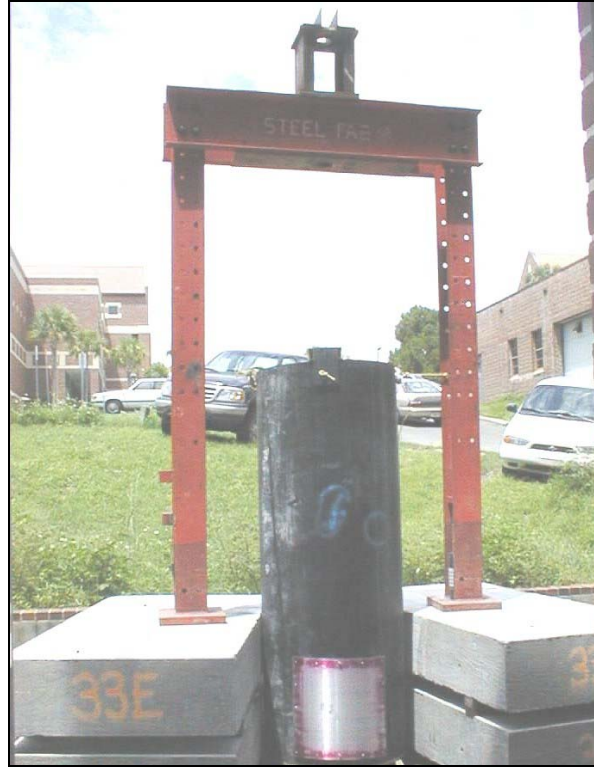
Figure 5.2 Exterior View of DTP Calibration Chamber
