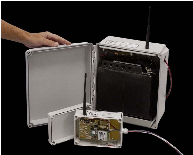
Figure 5. The MCPS enclosures are shown. The large enclosure is a Remote Monitoring Unit. It should be located on the structure that will receive the cathodic protection application. The smaller enclosure is a Base Reporting Unit. It should be located as near as possible to a data acquisition unit, data logger or other data storage or long-distance transmission device.
