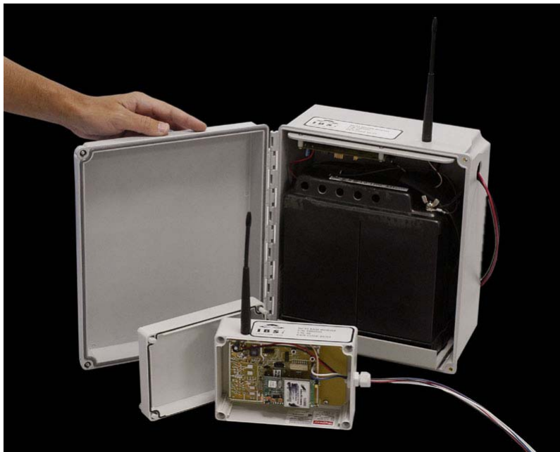
Figure 1. The MCPS enclosures are shown. The large enclosure is a Remote Monitoring Unit containing two batteries, CP application and monitoring electronics module mounted above them and an RF antenna attached to the top. The smaller enclosure is a Base Reporting Unit containing the same electronics module and an RF antenna attached to the top.
