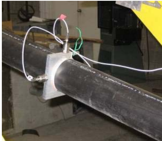
Figure 1.5 - Special accelerometer configuration for Tendon 13B.
