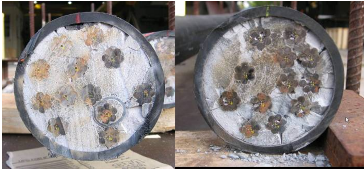
Figure 1.9 - Tendon 0A. L: Near S end. R: Near N end. PVC pipe outline visible at S end. Mark denotes top of tendon. in this and subsequent pictures.
