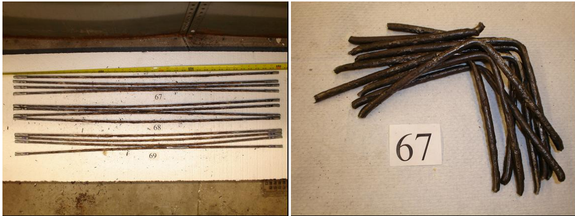
Figure 7.45 Retrieved Strands and Ties From #67, #68 and #69
