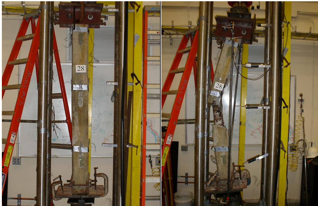
Figure 7.22 Failure of Unwrapped Control #28
