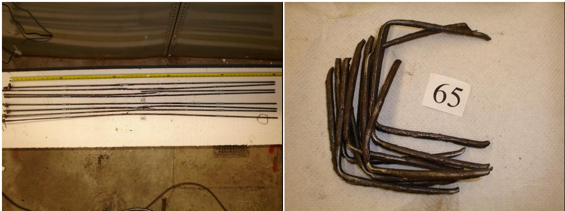
Figure 7.43 Retrieved Strands and Ties From #65 and #66
