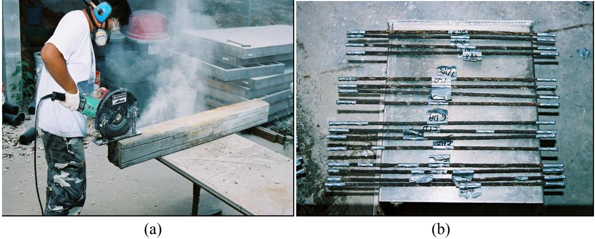
Figure 5.13 (a) Cutting Surface Concrete; (b) Retrieved Strands
