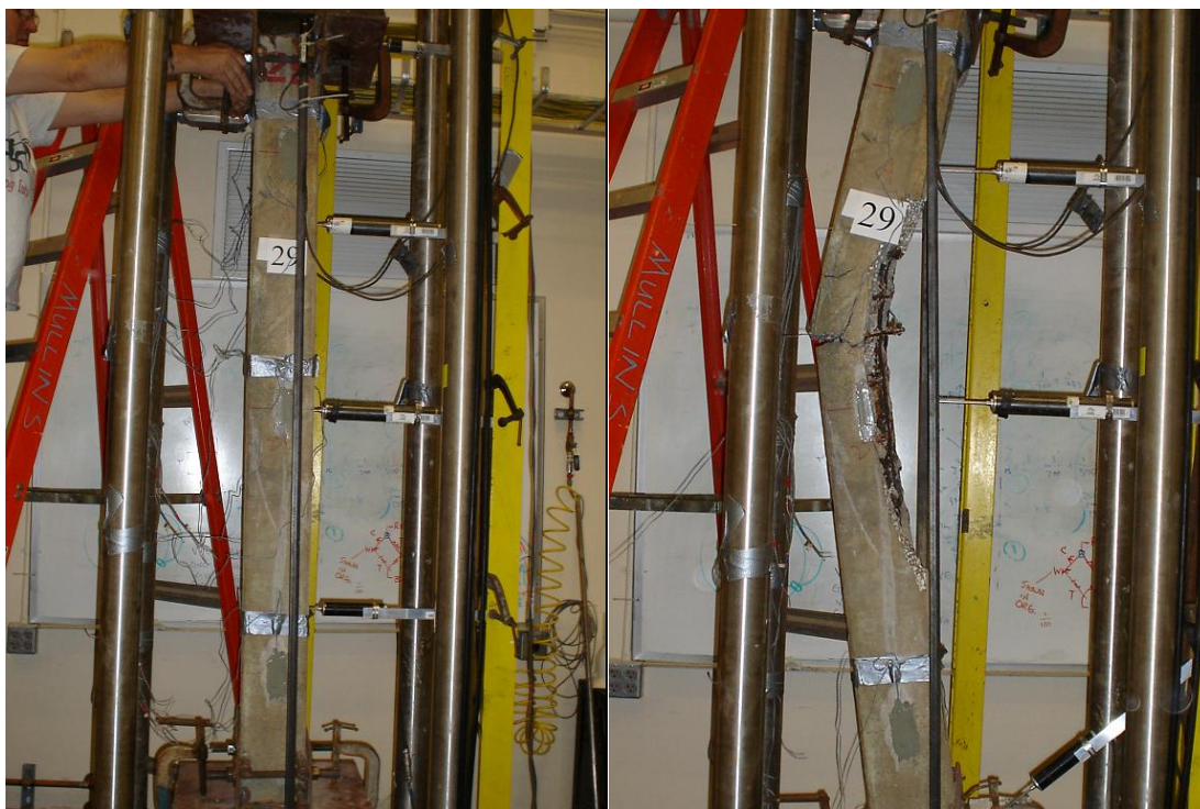
Figure 7.23 Failure of Unwrapped Control #29
