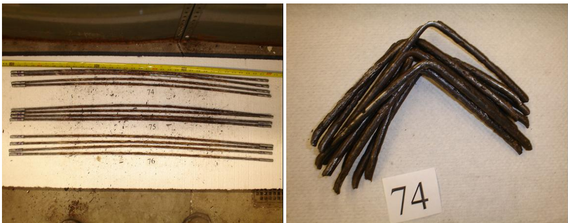
Figure 7.49 Retrieved Strands and Ties From #70, #71 and #72
