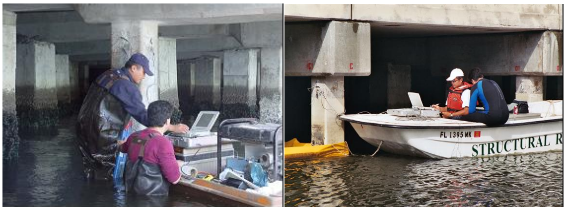
Figure 9.9 Performing Linear Polarization Measurement
