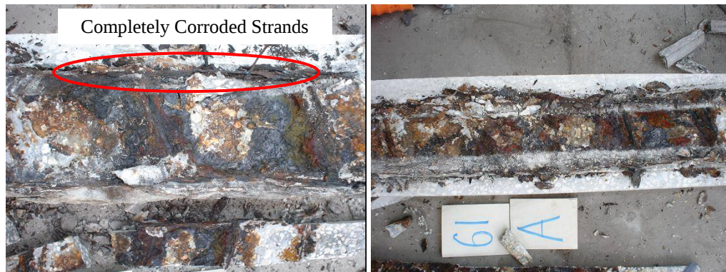
Figure 7.38 Distribution of Corrosion Product in #60 (L) and #61 (R) Specimens
