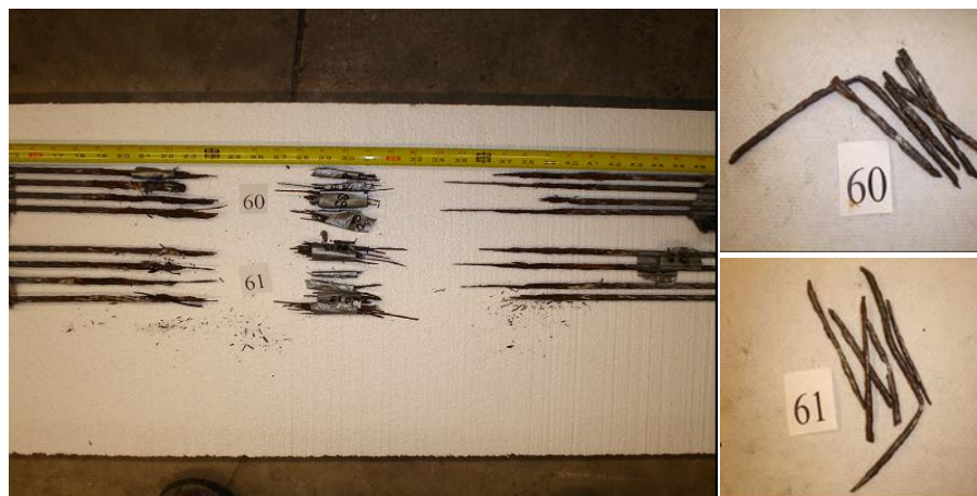
Figure 7.39 Retrieved Strands and Ties From Unwrapped Controls
