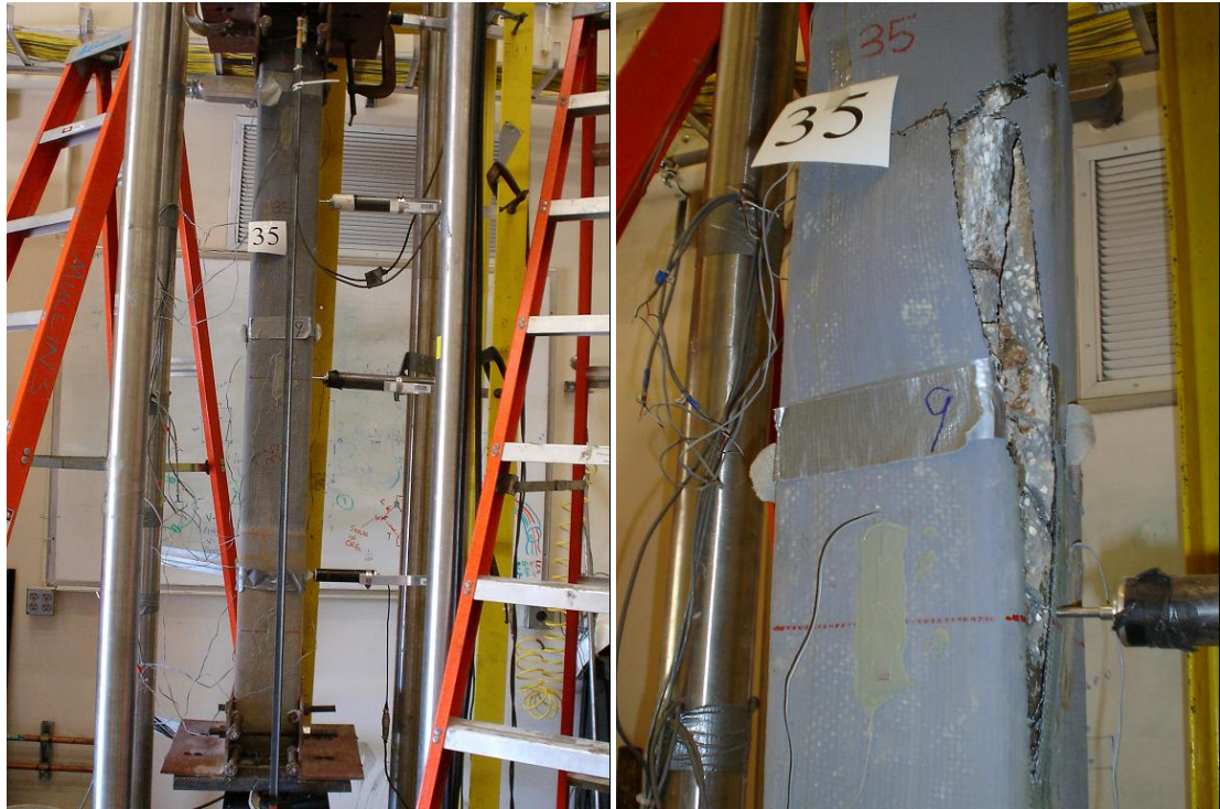
Figure 7.32 Failure of #35 Specimen (Minimal Repair, 72 in Wrap, Seal)
