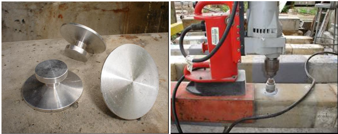
Figure 6.26 Aluminum Dollies (L) and Coring with a Diamond Drill Bit (R)
