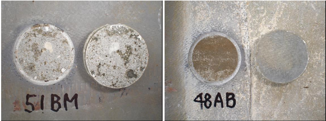
Figure 6.29 Concrete Failure (L) and Epoxy Failure Between Fiber and Concrete Surface in GFRP Wrapped Specimens (R)
