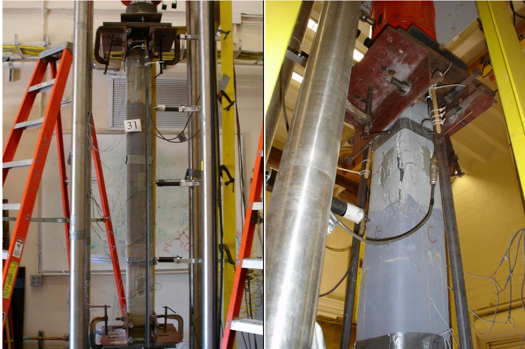
Figure 7.26 Failure of Specimen #31 (Full Repair, 36 in. Wrapped, Sealed)
