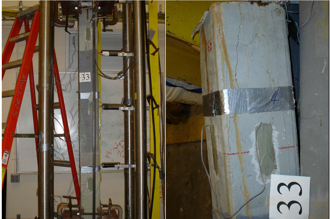
Figure 7.29 Failure of #33 Specimen (Minimal Repair, 36 in Wrap, Seal)
