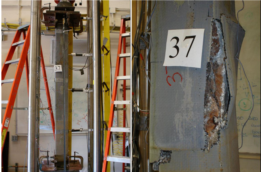
Figure 7.34 Failure of #37 Specimen (Minimal Repair, 72 in Wrap, Unseal)
