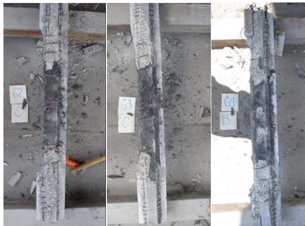
Figure 7.40 Distribution of Corrosion Product in #62 (L), #63 (M) and #64 (R)
