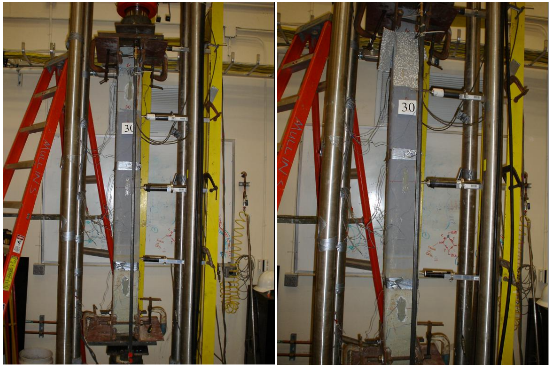
Figure 7.25 Failure of Specimen #30 (Full Repair, 36 in Wrapped, Sealed)
