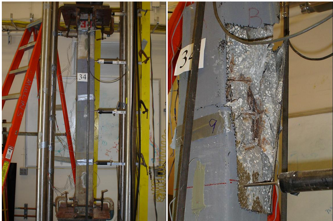
Figure 7.30 Failure of #34 Specimen (Minimal Repair, 36 in Wrap, Unseal)
