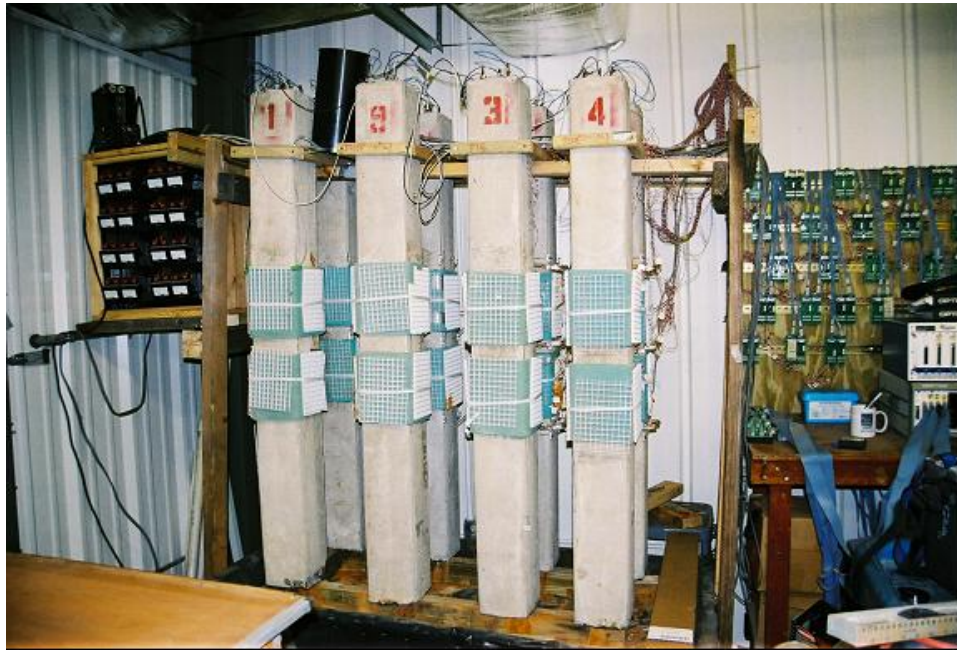
Figure 5.1 “Dry” Accelerated Corrosion Set Up.
