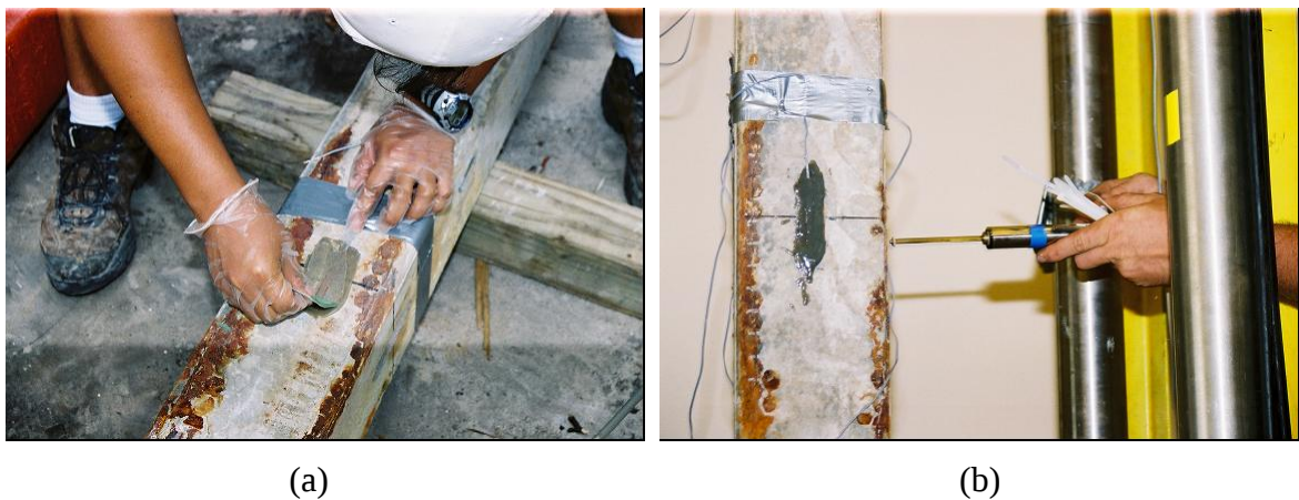
Figure 8.16 (a) Installing Strain Gages; (b) Installing LVDT
