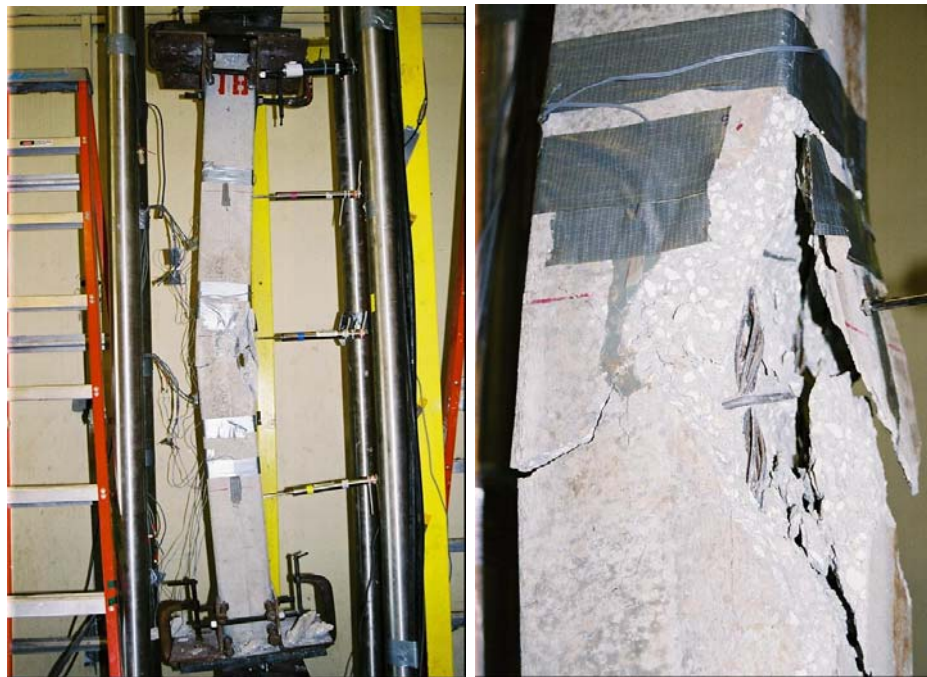
Figure 8.17 Failure of Unwrapped Controls at 0% Steel Loss
