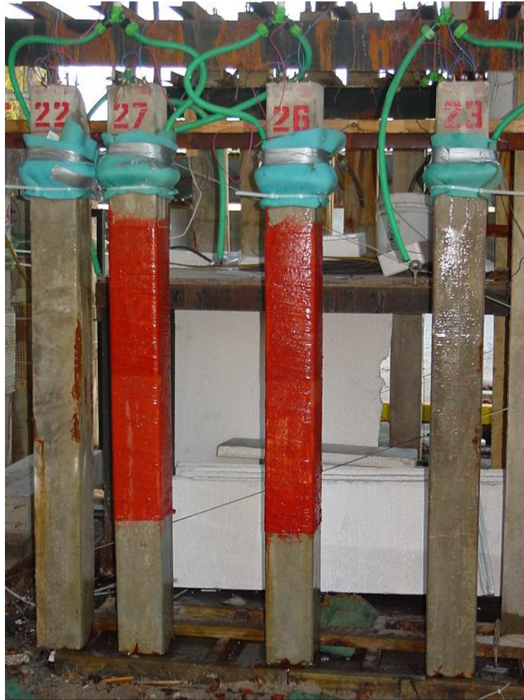
Figure 8.9 Corrosion Acceleration Set-up after Wrapping
