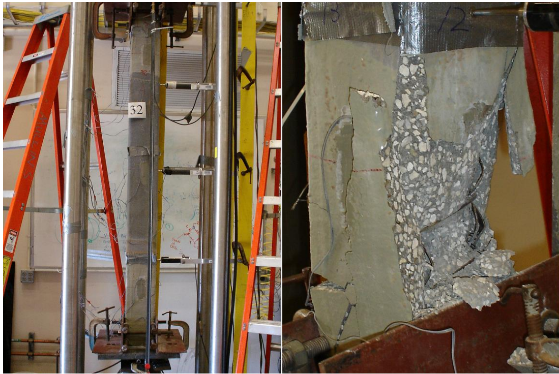
Figure 7.28 Failure of #32 Specimen (Minimal Repair, 36 in Wrap, Seal)
