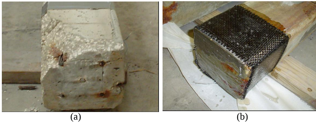
Figure 8.15 (a) Damaged End; (b) Repaired End
