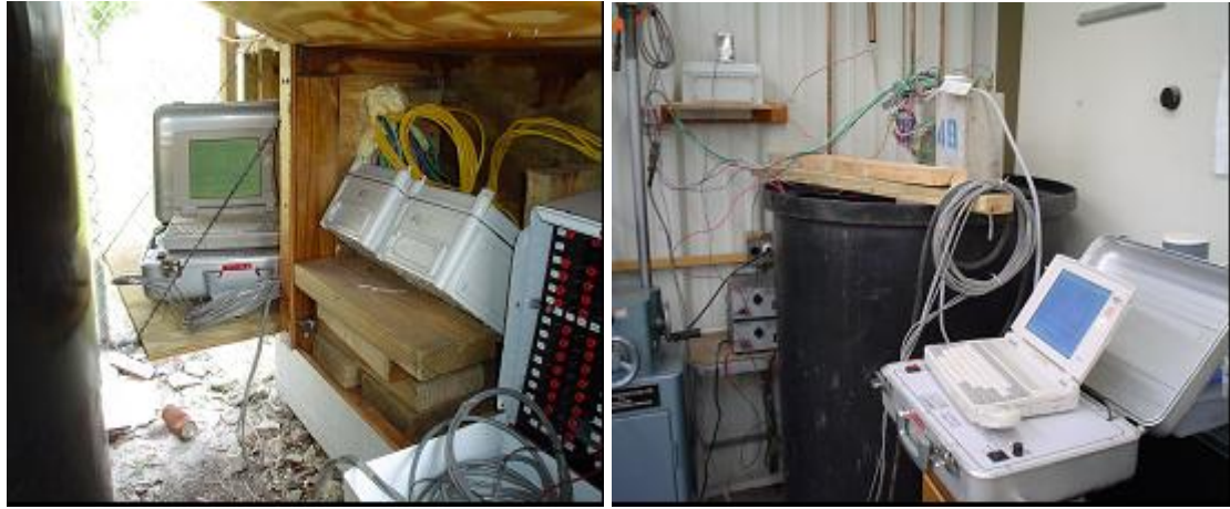
Figure 6.4 Linear Polarization Measurement Using PR Monitor
