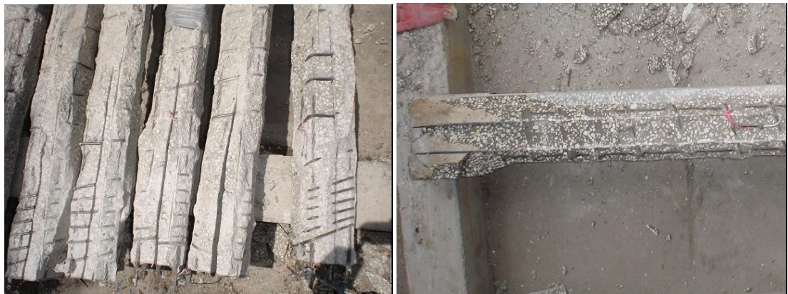
Figure 6.35 Lower Area of Wrapped Specimen Exposed to Wet/Dry Cycles
