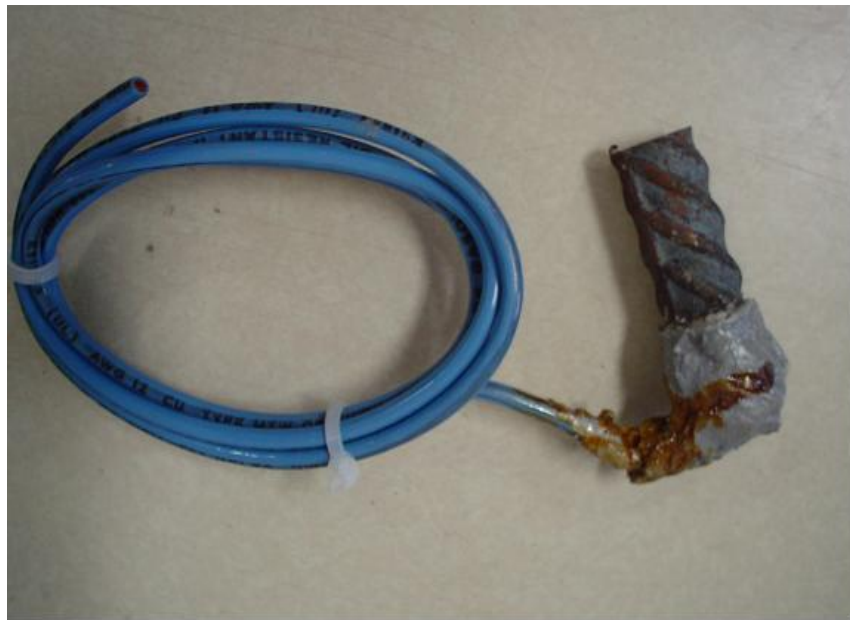
Figure 10.7 Rebar Probe Developed by FDOT
