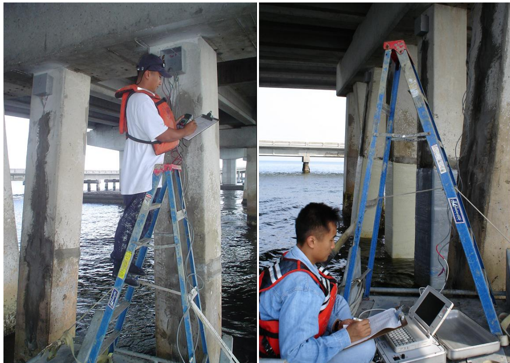
Figure 10.23 Current Flow Measurement (L) and Linear Polarization Test (R)
