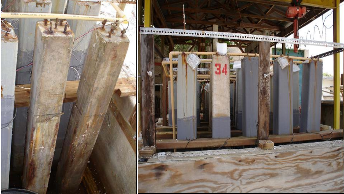
Figure 7.17 Unwrapped (L) and Wrapped (R) Specimens After the Exposure
