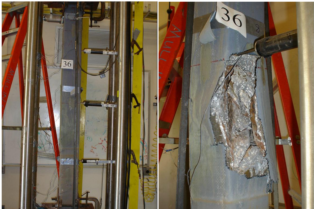
Figure 7.33 Failure of #36 Specimen (Minimal Repair, 72 in Wrap, Seal)
