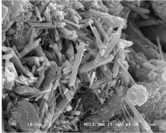
Figure 34. Ettringite Appearance in PP Cement
