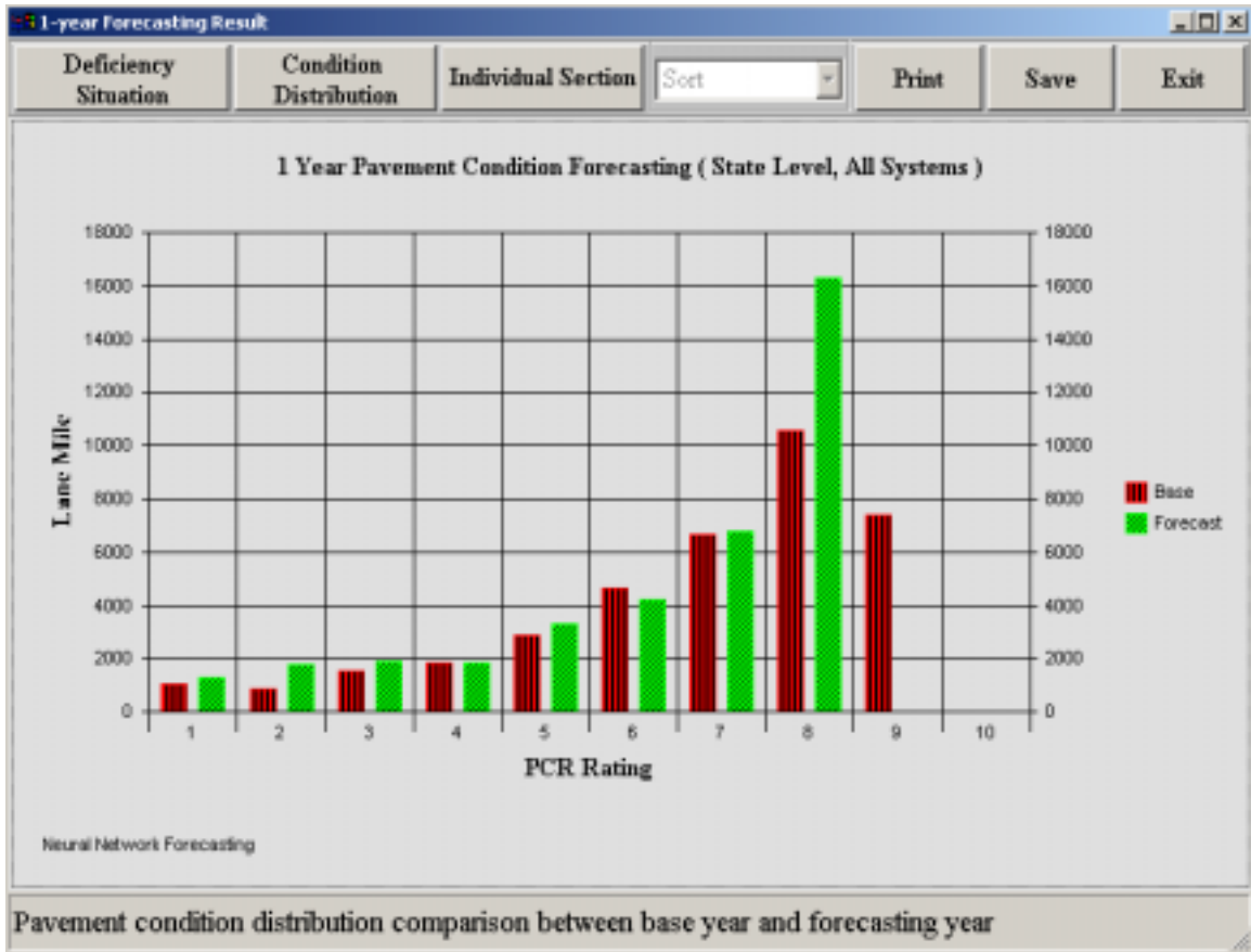
Figure 7.6 Distribution of Overall Pavement Condition
