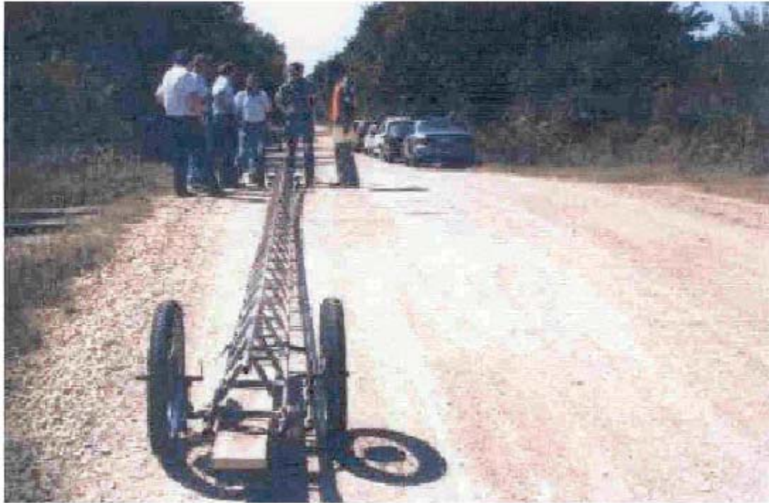
Figure 1.6. End View of Kansas Study's Physical Model for Measuring Hang-up [Mutabazi and Russell 2003]
