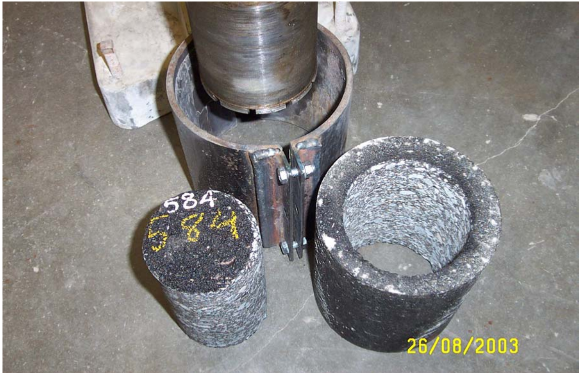
Figure 4-9. Coring of the Superpave Specimen
