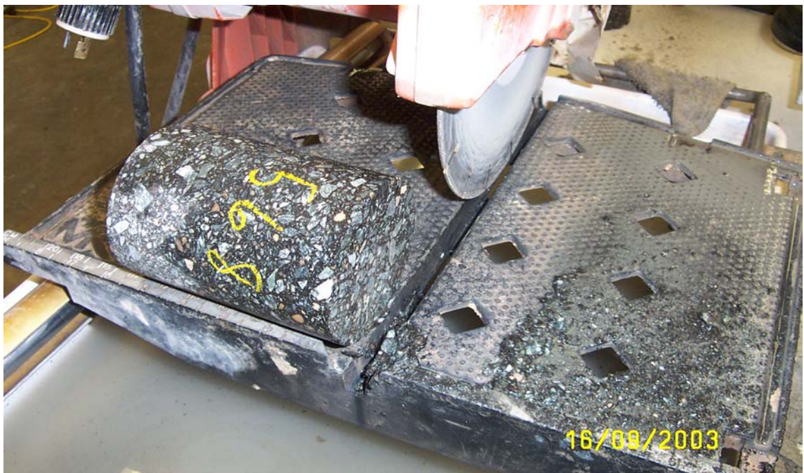
Figure 4-10. Cutting of the Dynamic Modulus Specimen
