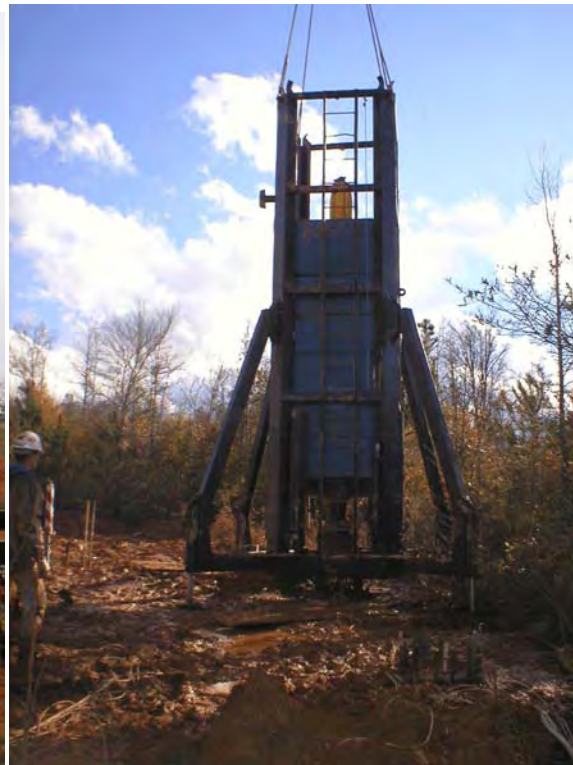
Figure 4-68 NGES Auburn: USF & FHWA's 4 MN Statnamic hydraulic catching device.
