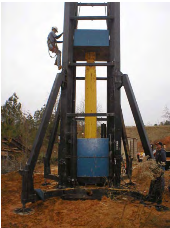
Figure 4-68 NGES Auburn: USF & FHWA's 4 MN Statnamic hydraulic catching device.
